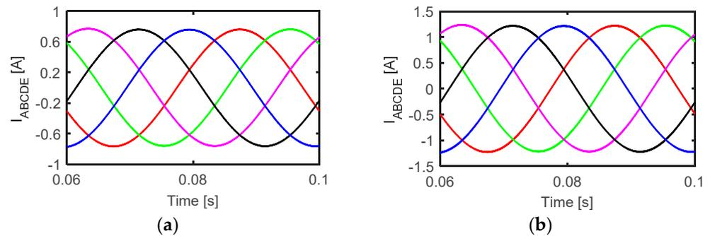
**Figure 12.** Simulation results of the output phase currents at unity modulation index and 25 Hz for (a) 2L + 2M and (b) 6L methods.
