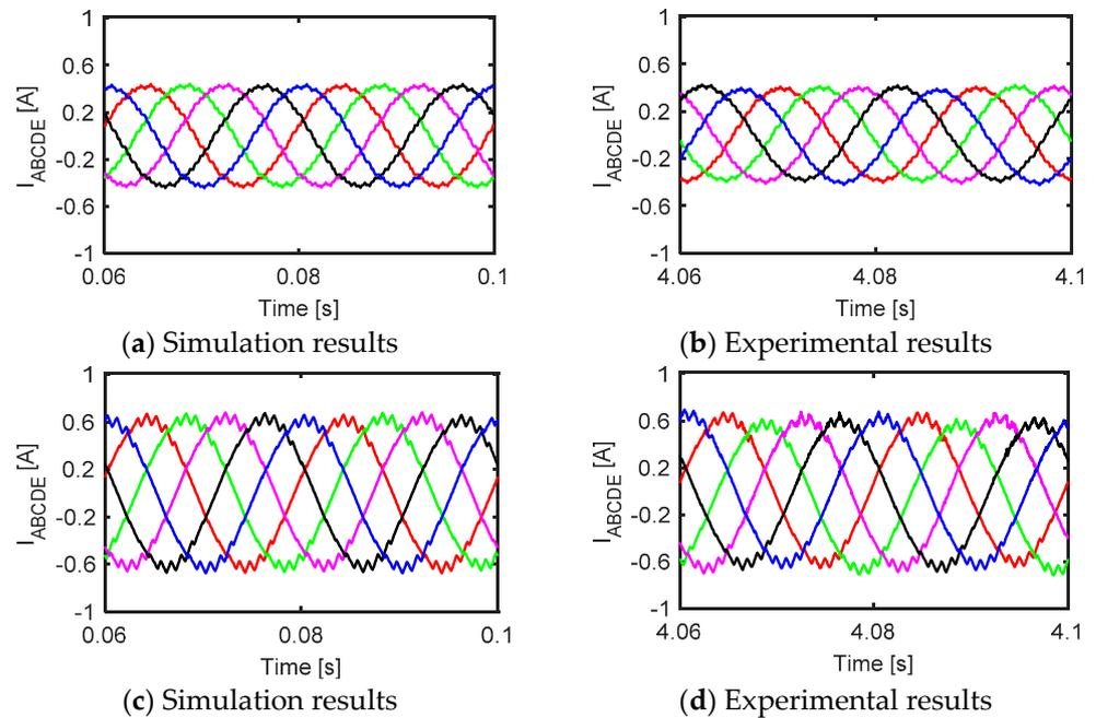
**Figure 20.** Experimental and simulation results of the output phase currents at unity modulation index and 50 Hz: (a) simulation results of 2L + 2M method, (b) experimental results of 2L + 2M method, (c) simulation results of 6L method, and (d) experimental results of 6L method.
