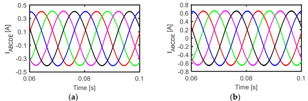
**Figure 9.** Simulation results of the output phase currents at unity modulation index and 50 Hz for (a) 2L + 2M and (b) 6L methods.
