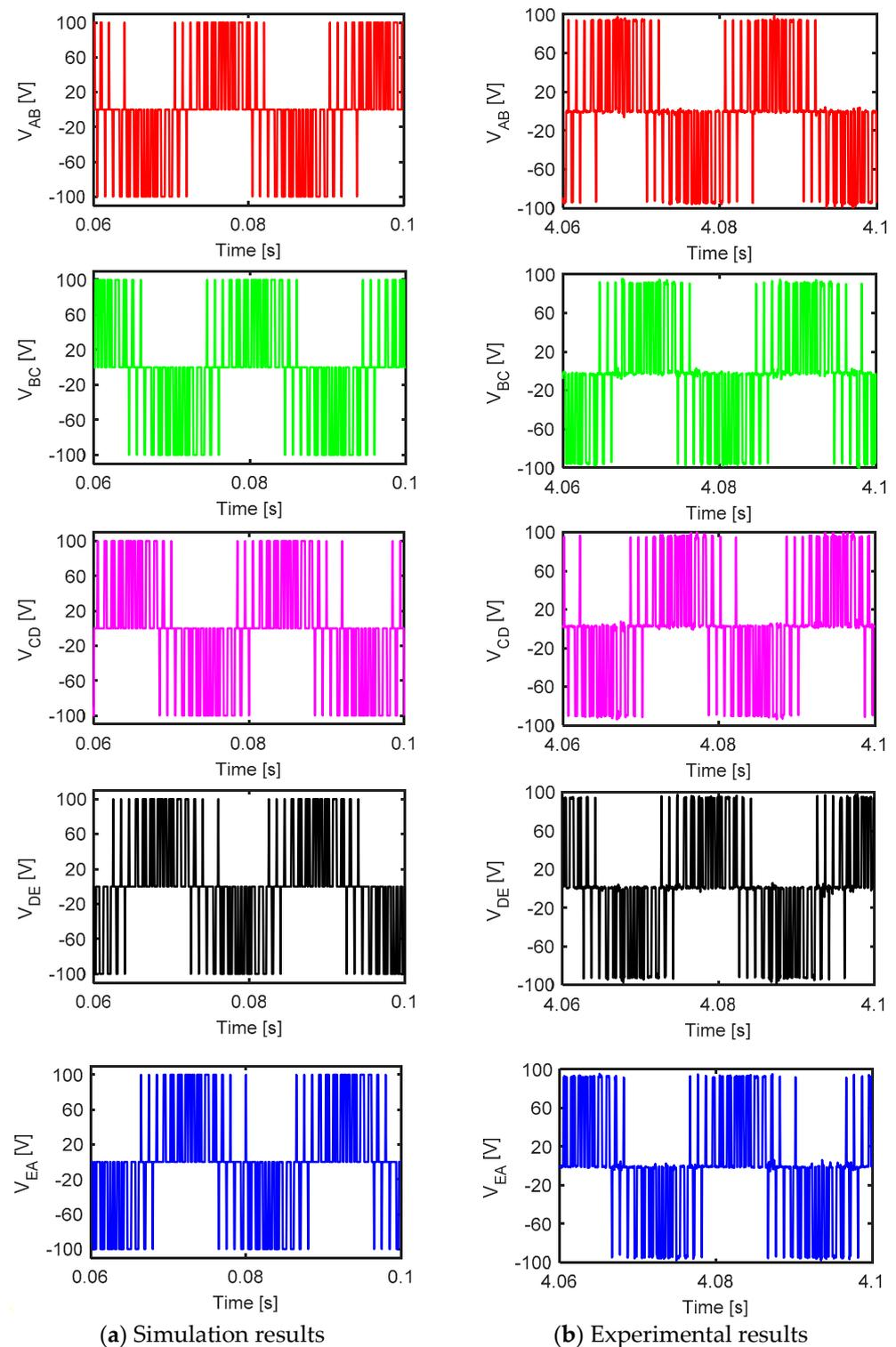
**Figure 19.** Experimental and simulation results of the output line-to-line voltages at unity modulation index and 50 Hz for 6L method's (a) simulation results and (b) experimental results.
