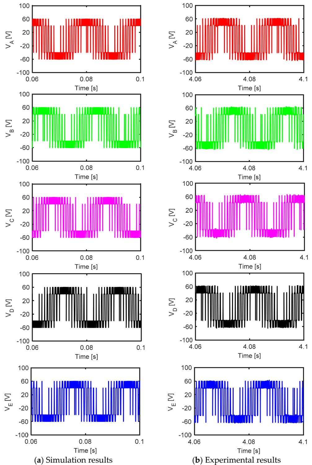
**Figure 17.** Experimental and simulation results of the output phase voltages at unity modulation index and 50 Hz for 6L (a) simulation and (b) experiment.
