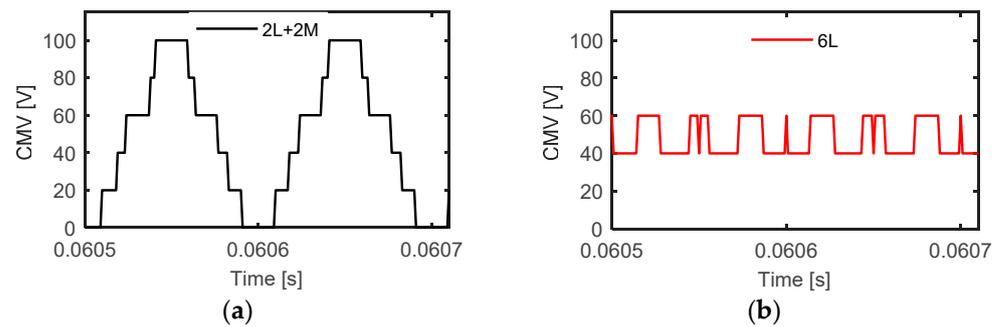
**Figure 6.** Simulation results of the CMV at unity modulation index and 50 Hz for (a) 2L + 2M and (b) 6L methods.
