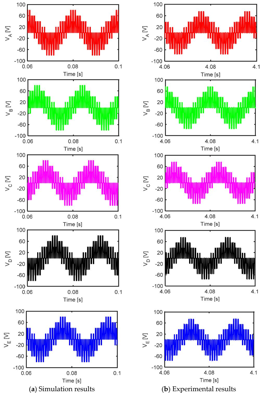
**Figure 16.** Experimental and simulation results of the output phase voltages at unity modulation index and 50 Hz for 2L + 2M (a) simulation and (b) experiment.
