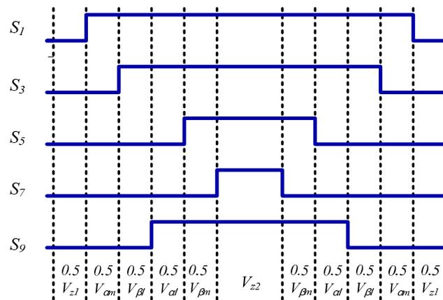
**Figure 3.** The 2L + 2M switching pattern for the top switches of the five-phase VSI in the first sector.
