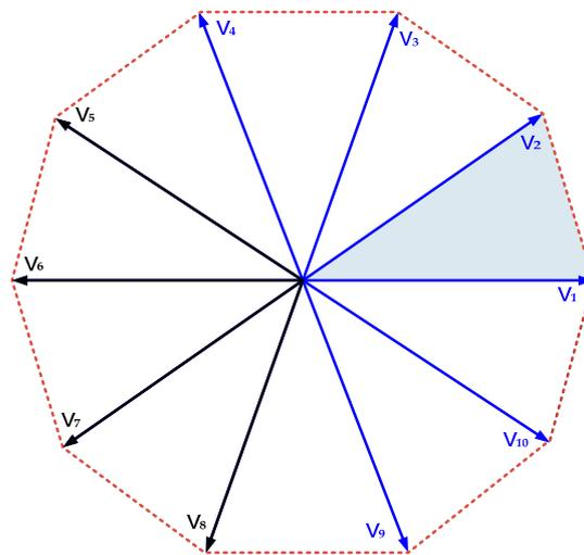
Figure 4. The 6L switching pattern in the  $\alpha$ - $\beta$  plane.
