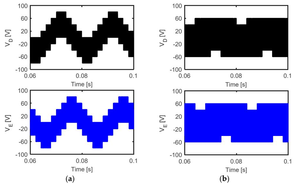
**Figure 7.** Simulation results of the output phase voltages at unity modulation index and 50 Hz for (a) 2L + 2M and (b) 6L methods.
