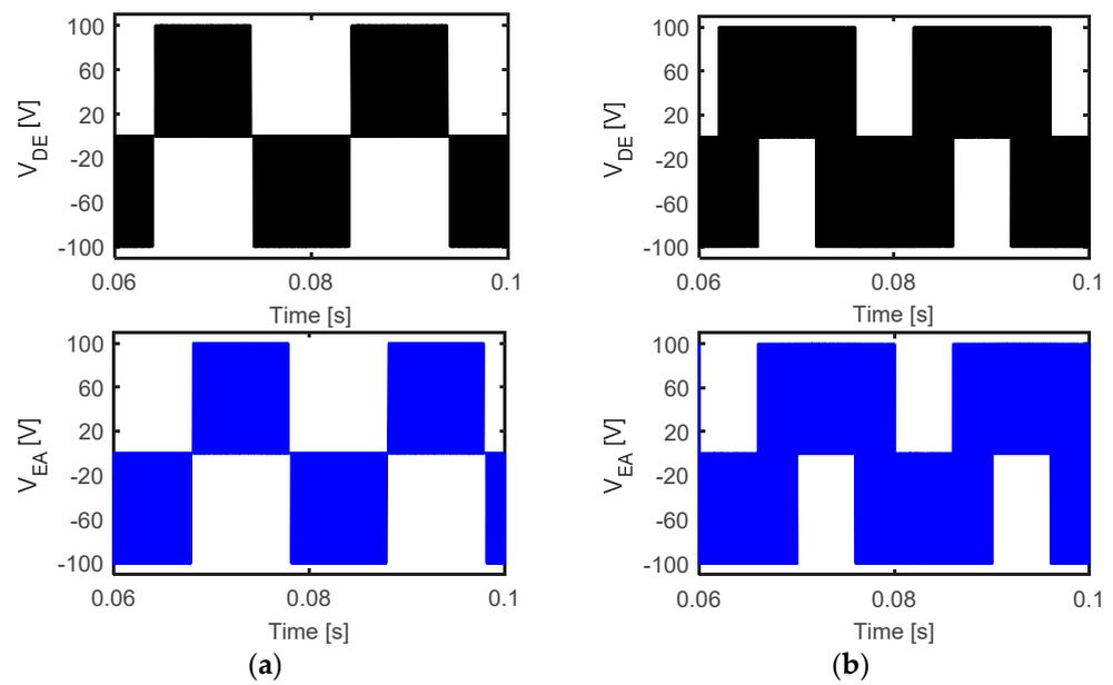
**Figure 8.** Simulation results of the output line-to-line voltages at unity modulation index and 50 Hz for (a) 2L + 2M and (b) 6L methods.
