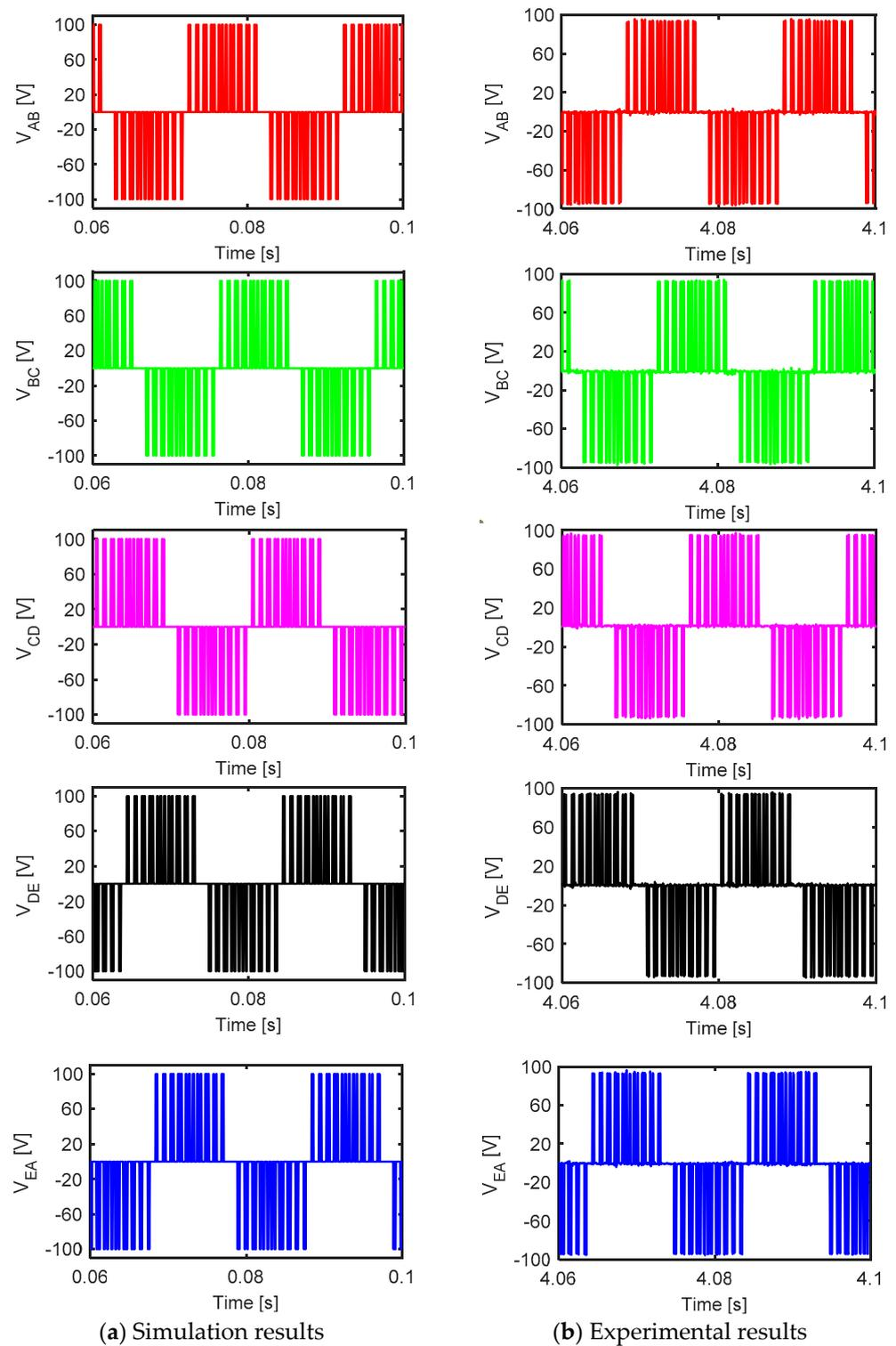
**Figure 18.** Experimental and simulation results of the output line-to-line voltages at unity modulation index and 50 Hz for 2L + 2M method's (a) simulation results and (b) experimental results.
