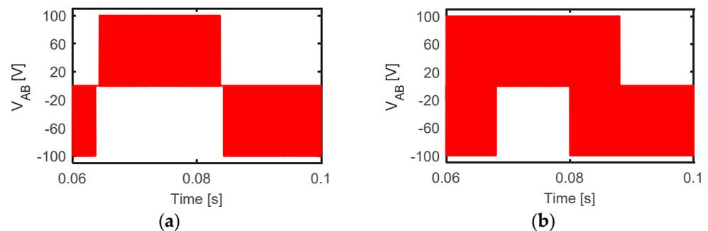
**Figure 13.** Simulation results of the output line-to-line voltage at unity modulation index and 25 Hz for (a) 2L + 2M and (b) 6L methods.
