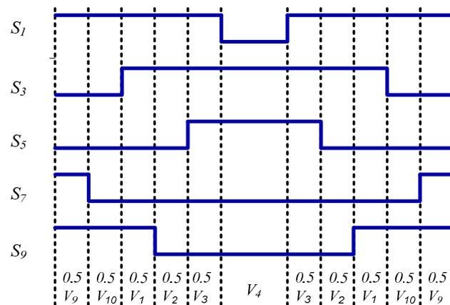
**Figure 5.** The 6L switching arrangement for the top switches of the five-phase VSI in the first zone.
