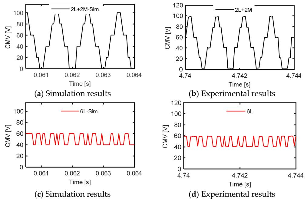
Figure 15. Experimental and simulation results of the CMV at unity modulation index and 50 Hz for (a) simulation of 2L + 2M method, (b) experiment of 2L + 2M method, (c) simulation of 6L method, and (d) experiment of 6L method.
