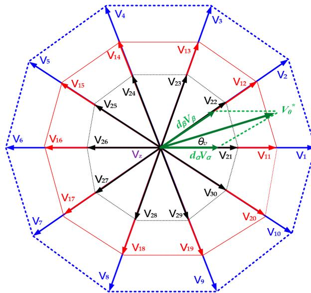
Figure 2. Switching voltage space vectors in the  $\alpha$ - $\beta$  plane.
