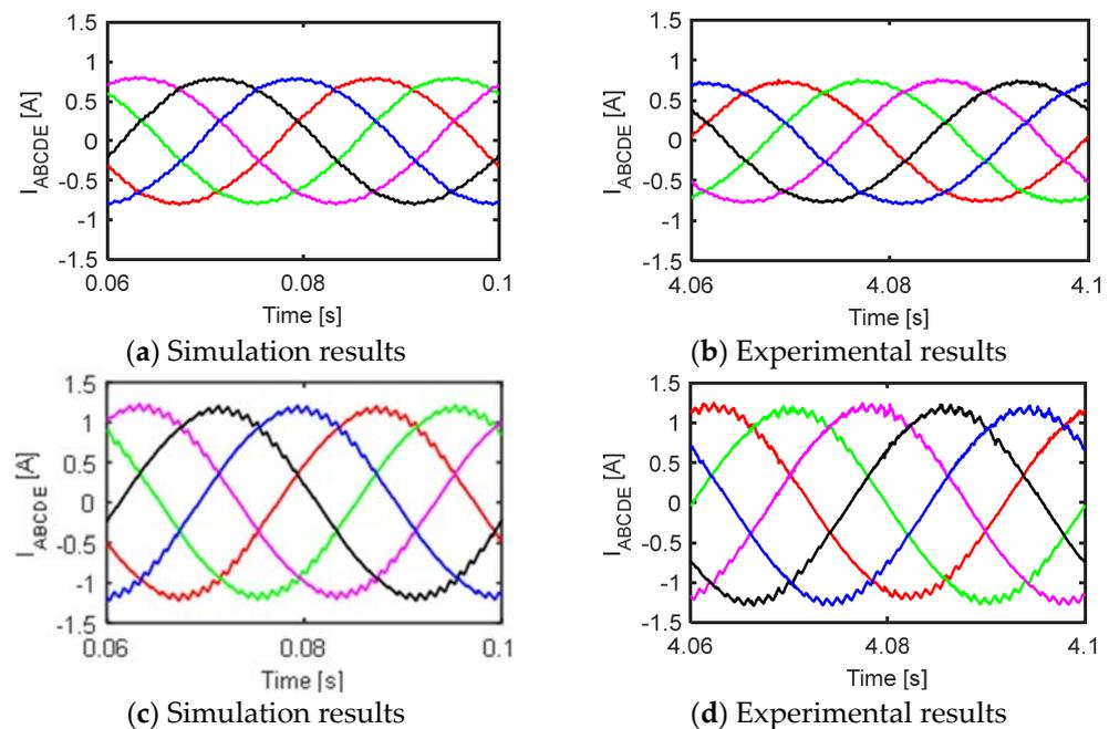
**Figure 21.** Experimental results of the output phase currents at unity modulation index and 25 Hz: (a) simulation results of 2L + 2M method, (b) experimental results of 2L + 2M method, (c) simulation results of 6L method, and (d) experimental results of 6L method.
