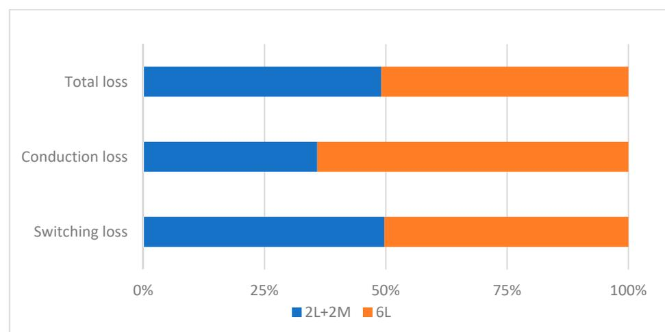
**Figure 11.** Simulation results of the inverter switching and conduction losses at unity modulation index and 50 Hz.
