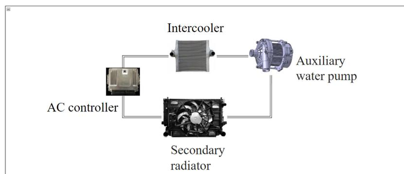
**Figure 6.** Schematic diagram of secondary cooling system in test system.
