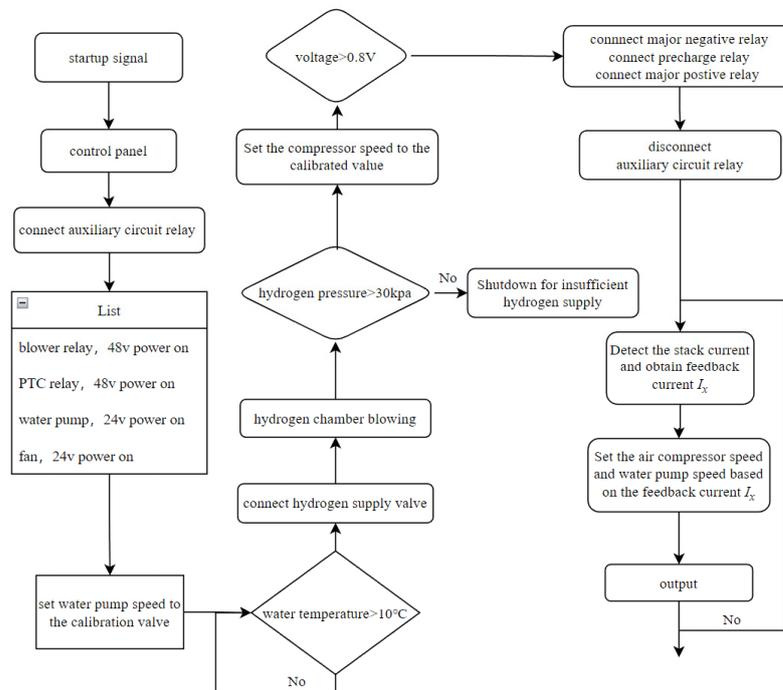
Figure 8. Power-on procedure.
