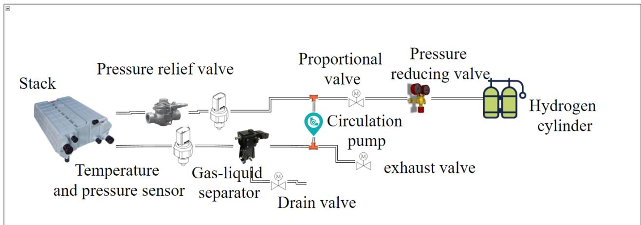
**Figure 3.** Schematic diagram of hydrogen supply subsystem in test system.
