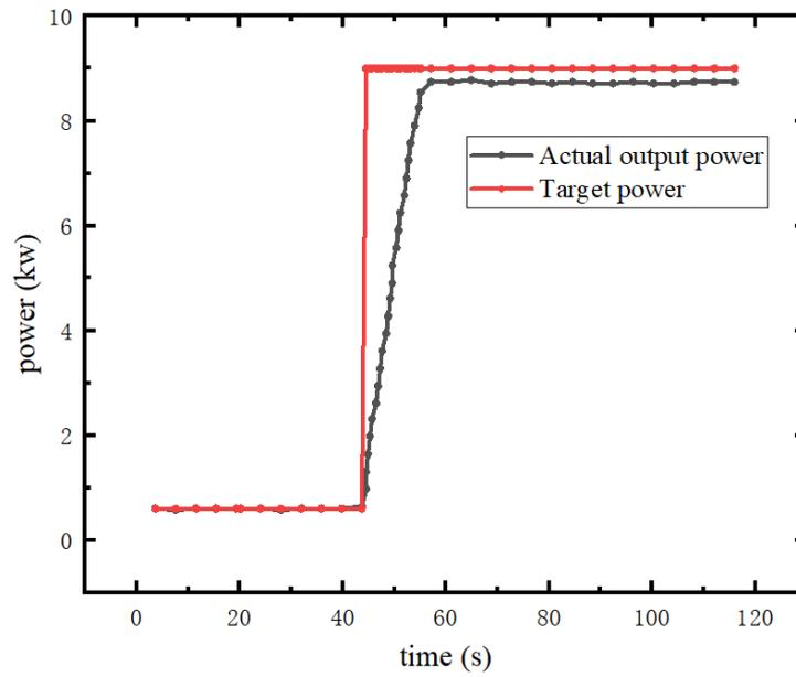
Figure 15. Dynamic response curve from idle to 90% rated power of the fuel cell.
