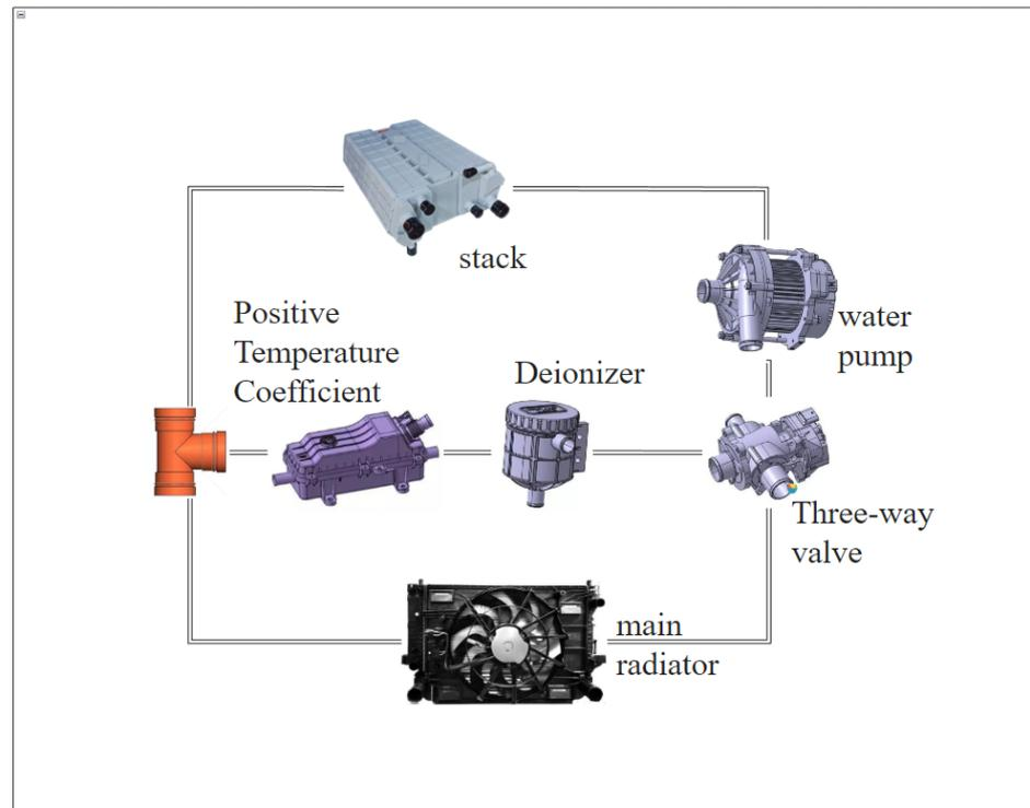
**Figure 5.** Schematic diagram of the main cooling system in the test system.
