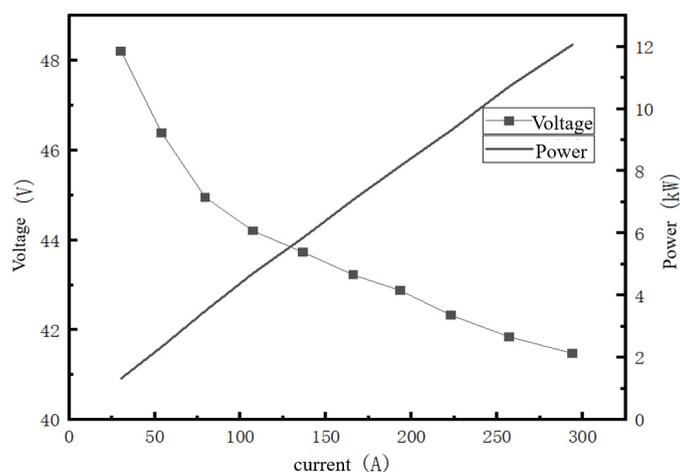
Figure 12. Variation curves of fuel cell output voltage and power with respect to current.
