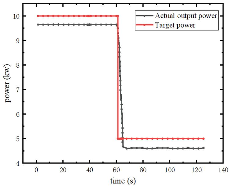
Figure 16. Response curve of rated power from unloaded to 50% of the fuel cell.
