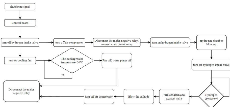
Figure 9. Power-off procedure.
