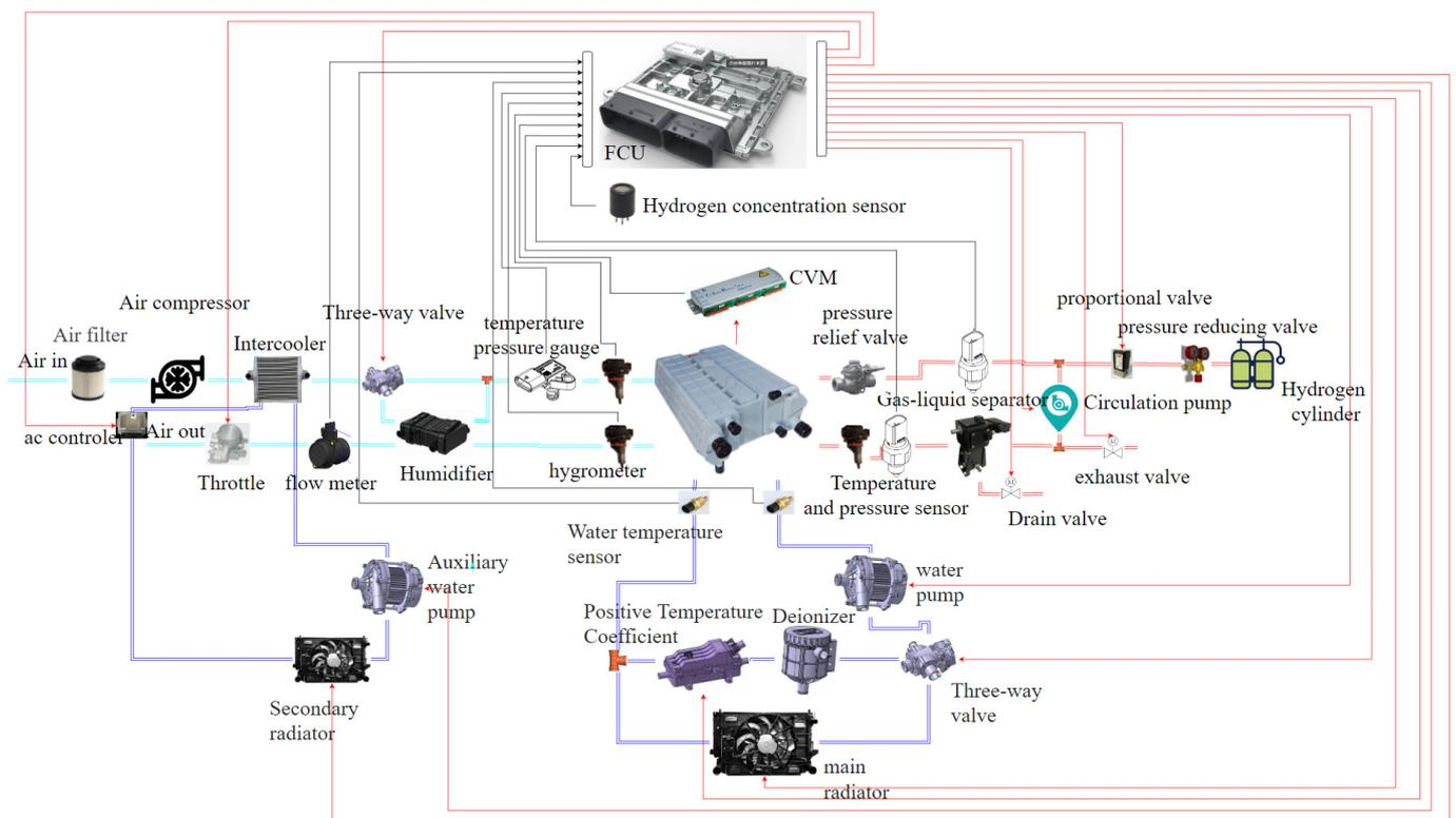
Figure 10. Schematic diagram of test system construction.
