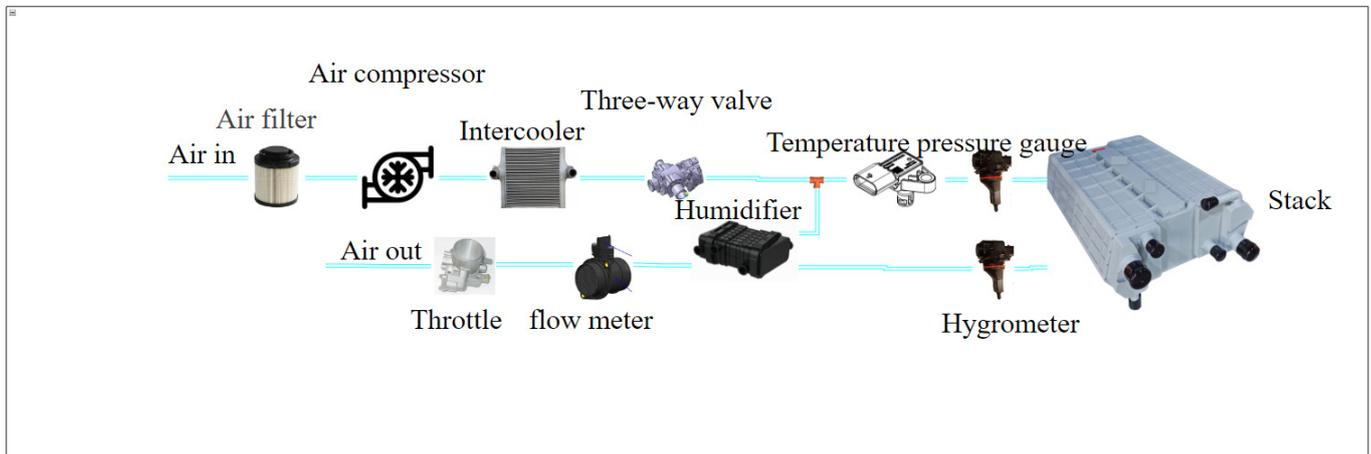
**Figure 4.** Schematic diagram of the air supply subsystem in the test system.
