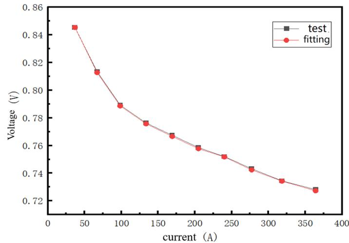
Figure 13. Variation curve of single cell average voltage with respect to current density.
