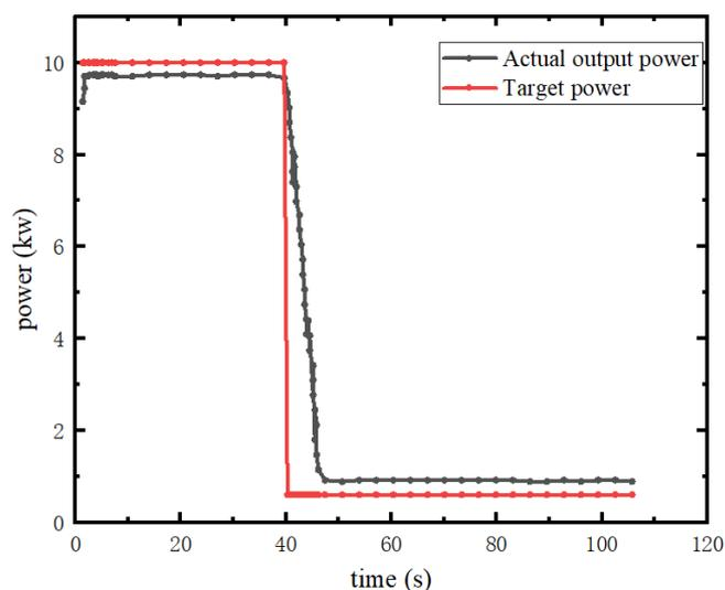
**Figure 17.** Response curve of rated power from unloaded to idle of the fuel cell.
