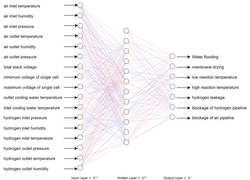
Figure 18. Neural network structure diagram.
