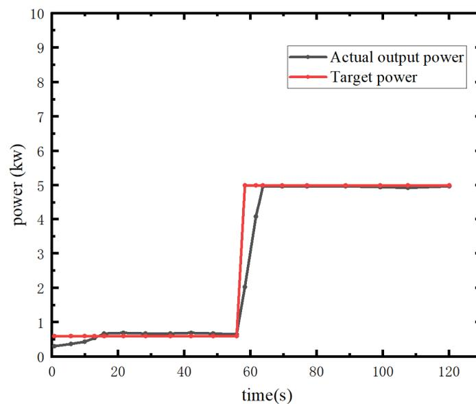
Figure 14. Dynamic response curve from idle to 50% rated power of the fuel cell.
