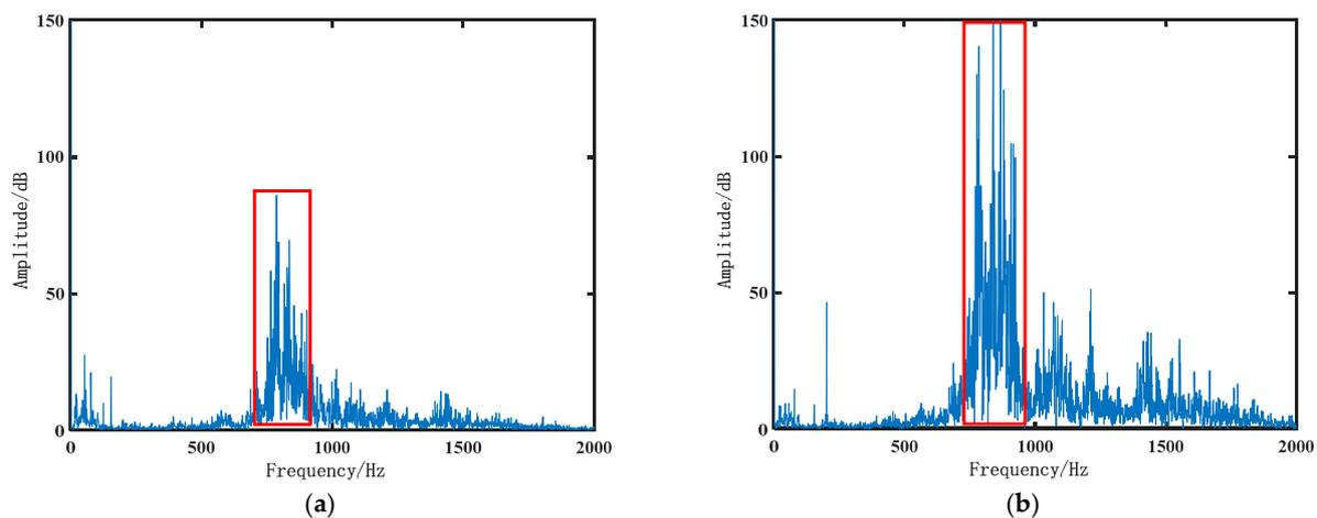
**Figure 6.** The spectrum of vibration signal obtained in the presence of thunderstorm noise: (a) switch closing process; (b) switch opening process.
