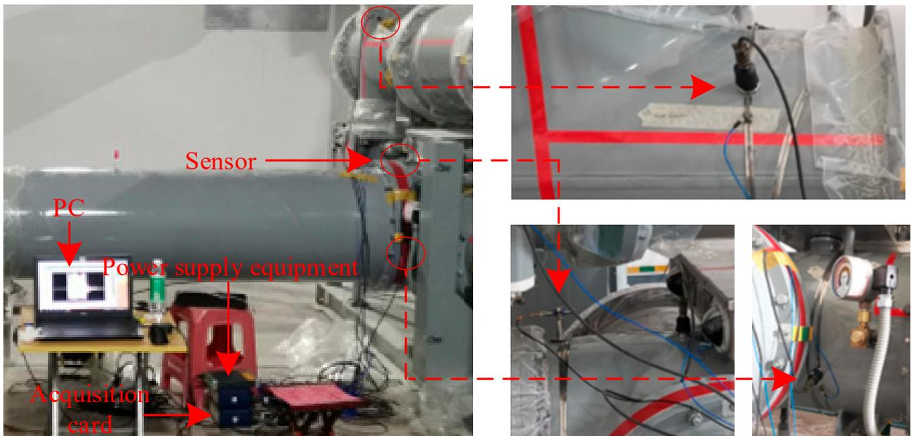
Figure 1. Photos of vibration detection system.
