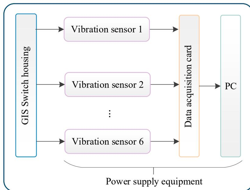
Figure 2. Block diagram of the vibration detection system.
