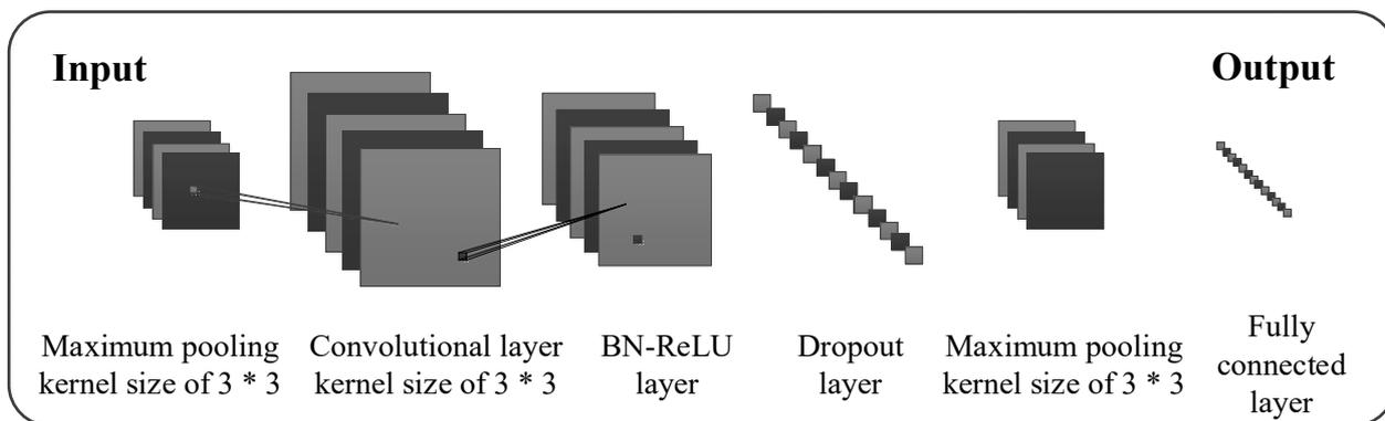
Figure 4. Block diagram of the FCNN method.
