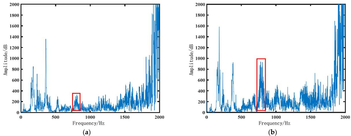
**Figure 5.** The spectrum of vibration signal obtained without background noise: (a) switch closing process; (b) switch opening process.
