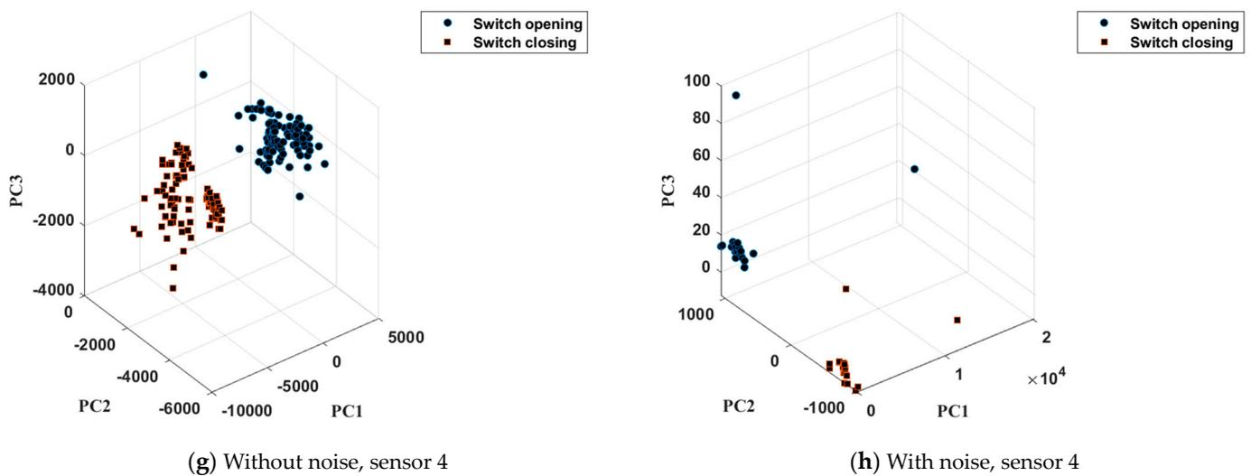
Figure 7. Feature distributions of vibration signal without noise and with thunderstorm noise.
