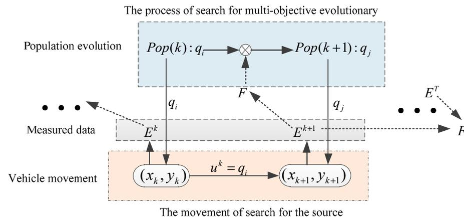
**Figure 4.** Diagram of the principle of source seeking.
