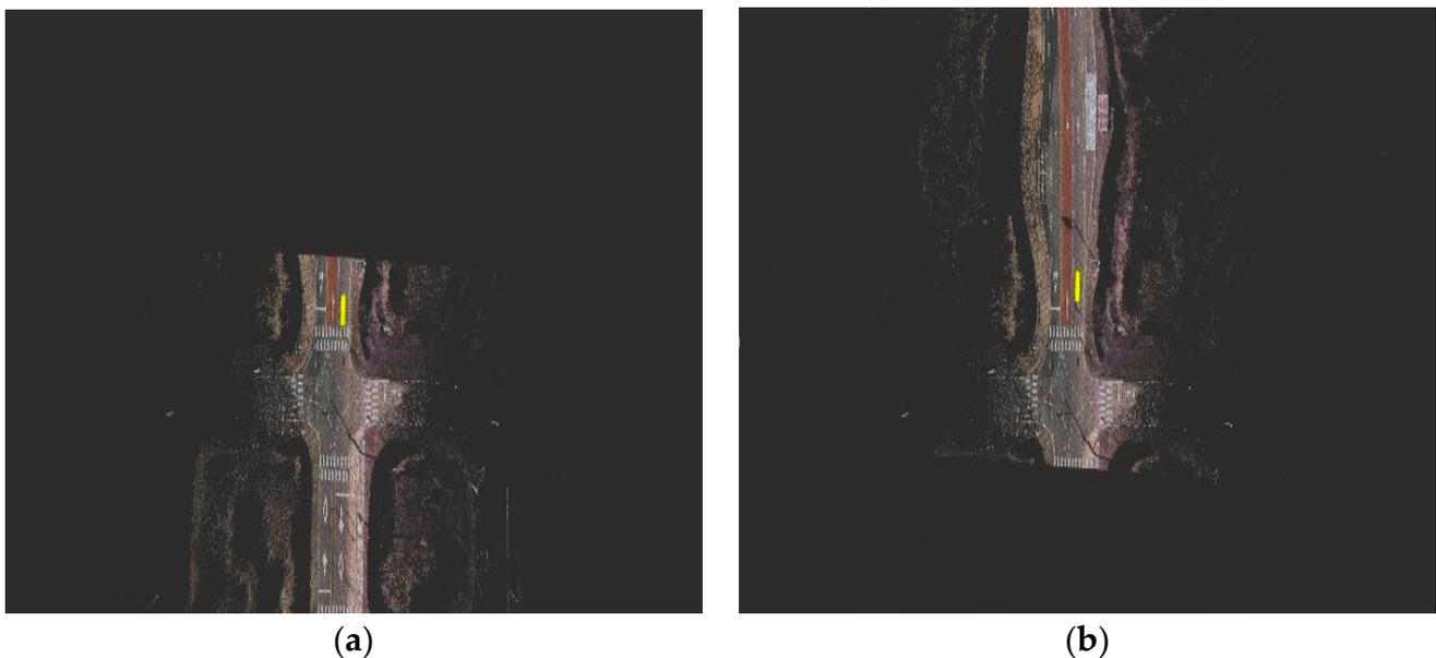
**Figure 8.** A sequence of images showing the localization process using a sub map received from infrastructure 1, in (a); and continuously downloading new sub maps in real time from infrastructure 2 in areas with stronger signals to perform localization, in (b).
