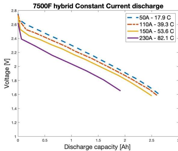
Figure 6. The 7500F hybrid constant current discharge curve.
