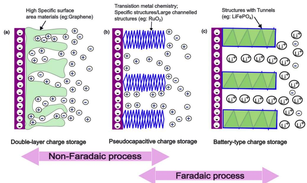
**Figure 2.** Electrode processes in: (a) electrical double layer, (b) pseudocapacitive, (c) Faradaic electrodes.
