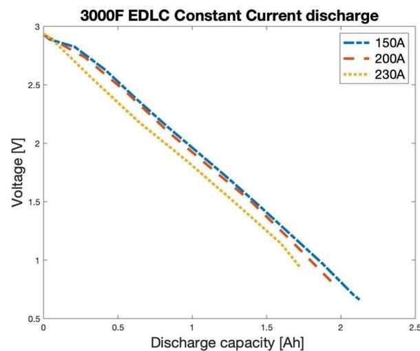
**Figure 5.** The 3000F EDLC constant current discharge.
