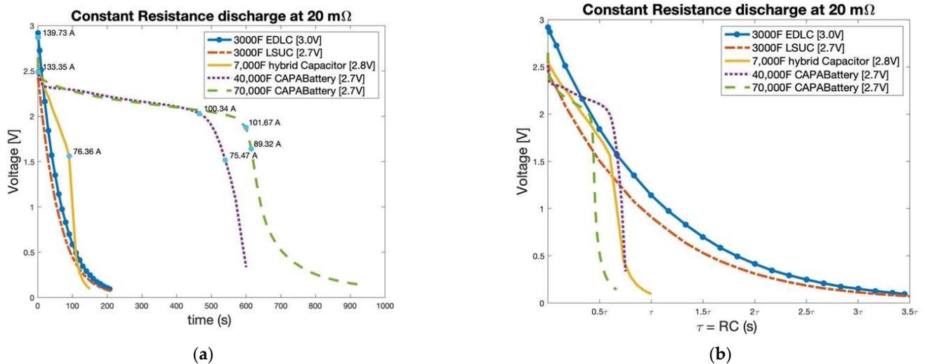
Figure 9. Constant resistance discharge curve: (a) with respect to time taken; (b) with respect to time constants.
