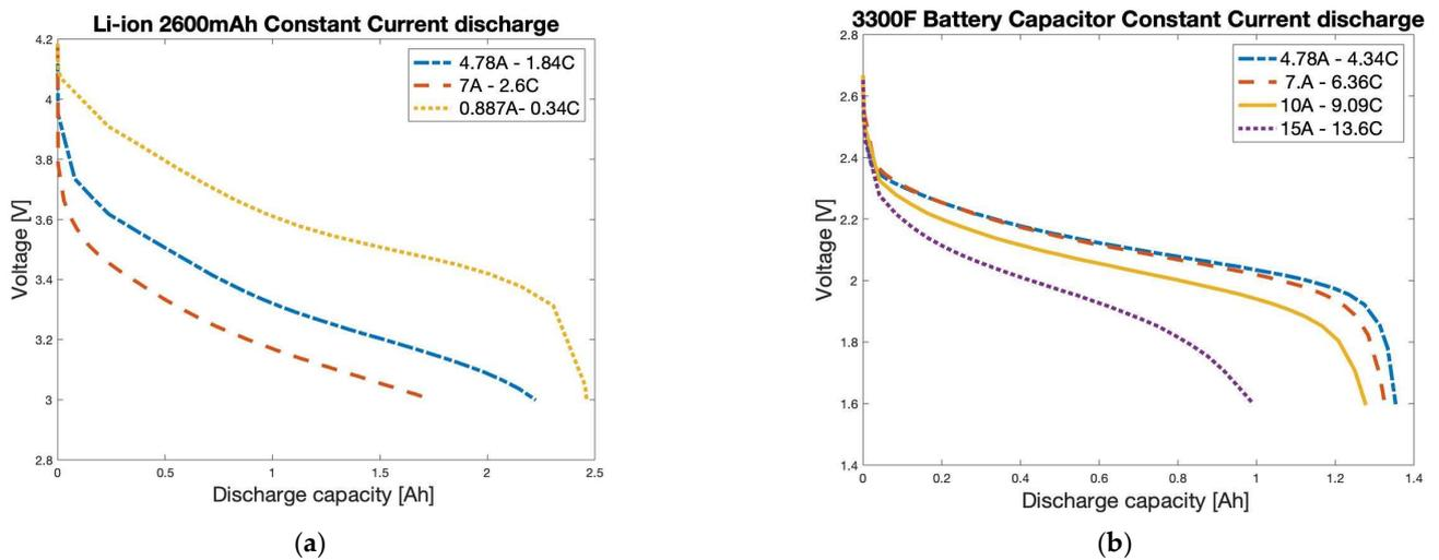
Figure 8. Constant current discharge curve (a) 18,650 Li-ion 2600 mAh; (b) 3300F battery capacitor.
