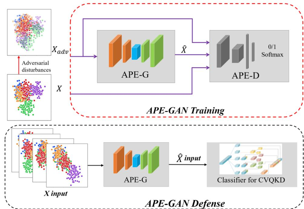
**Figure 4.** The frame of the APE-GAN based defense strategy.  $X$ : the original clean data.  $X_{adv}$ : Perturbed data after the adversarial attack.  $\hat{X}$ : the reconstructed data.
