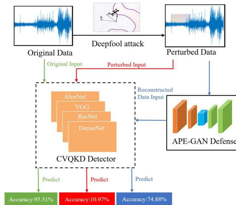
**Figure 5.** Schematic diagram of DeepFool attack and APE-GAN defense, where our chosen CNN classification models are AlexNet, VGG, ResNet, and DenseNet. The classification accuracy of the original data is 95.31% on average. Additionally, the average classification accuracy of perturbed data is 10.97% on average. The reconstructed data input achieves an accuracy of 74.88%.
