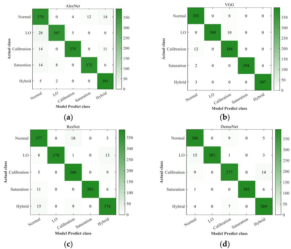
**Figure 3.** The confusion matrices of CNNs for CVQKD attack detection. (a) The AlexNet model classification results in five scenarios. (b) The VGG model classification results in five scenarios. (c) The ResNet model classification results in five scenarios. (d) The DenseNet model classification results in five scenarios.
