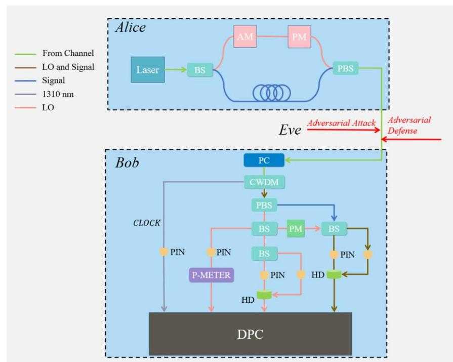
**Figure 1.** The schematic diagram for the attack detection portion of the CVQKD system considering adversarial attacks and defenses. The attack from Eve includes normal attacks and adversarial perturbations.
