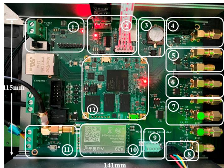
Figure 4. The actual picture of integrated offline data acquisition and control system for lidar.
