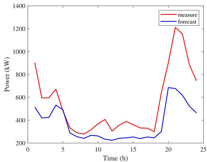
Figure 6. Forecast and actual of load profile data for peak day.
