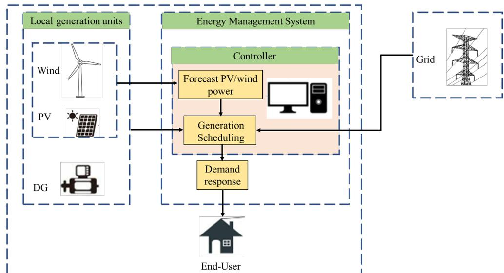
**Figure 1.** The proposed framework of the decentralized energy management system.
