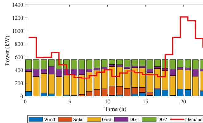
**Figure 8.** Case II: Microgrid generation scheduling for peak day with actual data.
