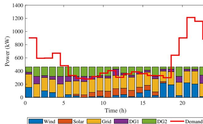
**Figure 9.** Case III: Microgrid generation scheduling for peak day with PV and wind forecast data and actual demand.
