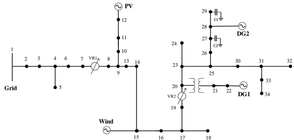
Figure 3. Microgrid test system [46].
