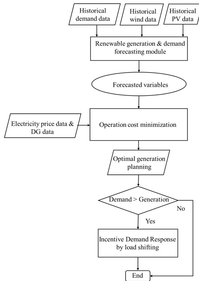
Figure 2. Flowchart for implementation of the proposed decentralized energy management system.
