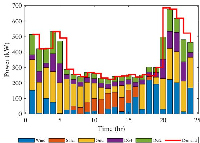
**Figure 7.** Case I: Microgrid generation scheduling for peak day with forecast data.
