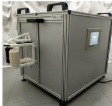
Figure 26. Textile yarn winding and unwinding machine.
