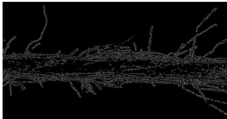
**Figure 36.** Insulated contours of the textile yarn.
