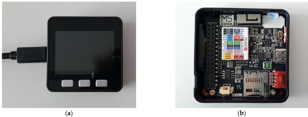
Figure 4. (a) M5 Stack Basic kit used for tests; (b) the kit opened, showing the ESP32.
