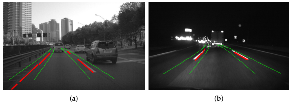
Figure 4. Line detection and lane tracking results: (a) daytime result, and (b) night result.
