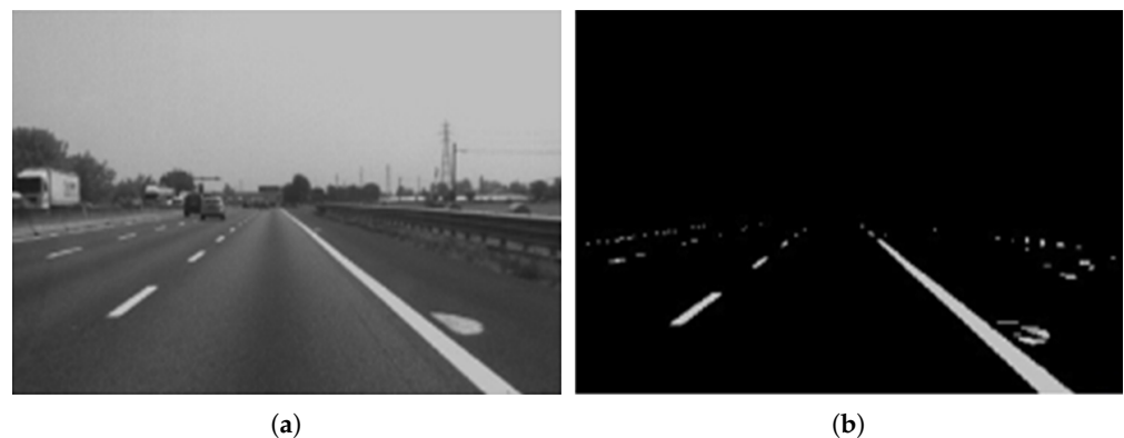
Figure 3. Dark-bright-dark filter result: (a) input image, and (b) dark-bright-dark filter result.
