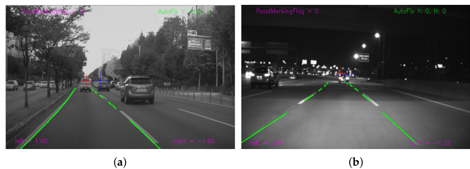
Figure 5. Line fitting results: (a) daytime result, and (b) night result.
