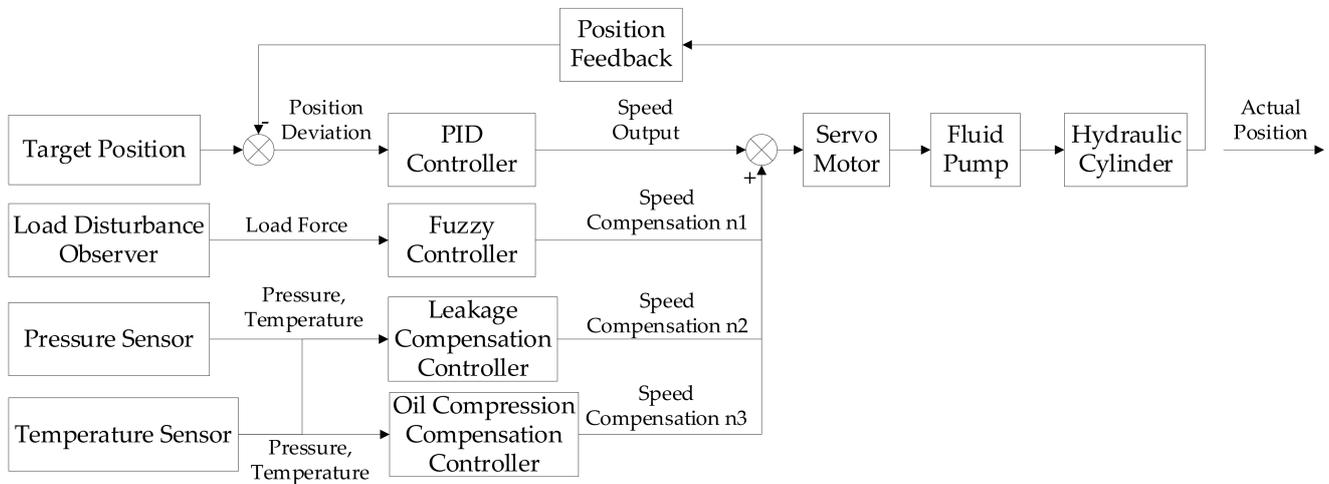
Figure 2. System control schematic diagram.
