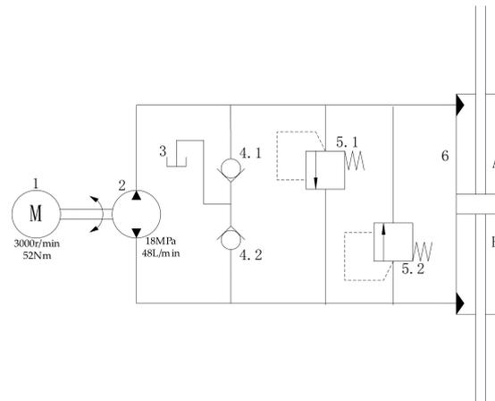
**Figure 1.** Hydraulic system diagram of electro-hydraulic servo pump control system: 1—servo motor; 2—quantitative pump; 3—hydraulic oil tank; 4—check valves; 5—relief valves; 6—hydraulic cylinder.
