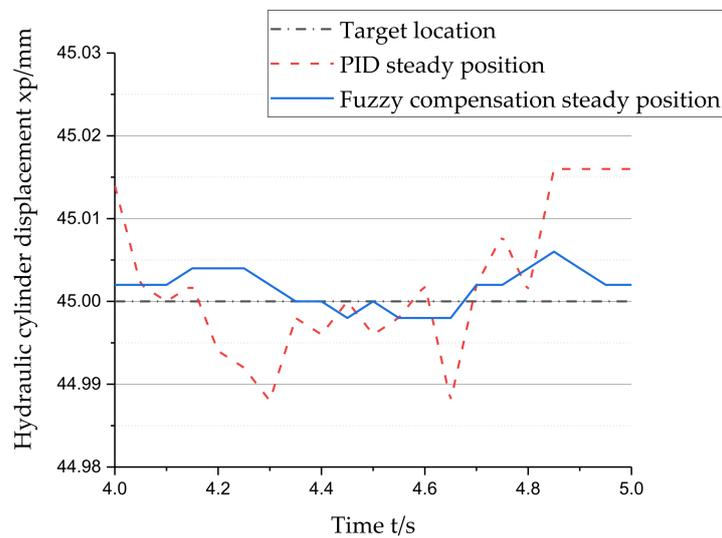
Figure 12. Local magnification curve of the retracted position of the hydraulic cylinder.
