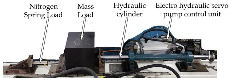
Figure 5. Hydraulic part of experimental platform.
