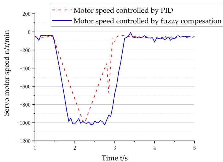
Figure 13. Speed response curve of the servo motor.
