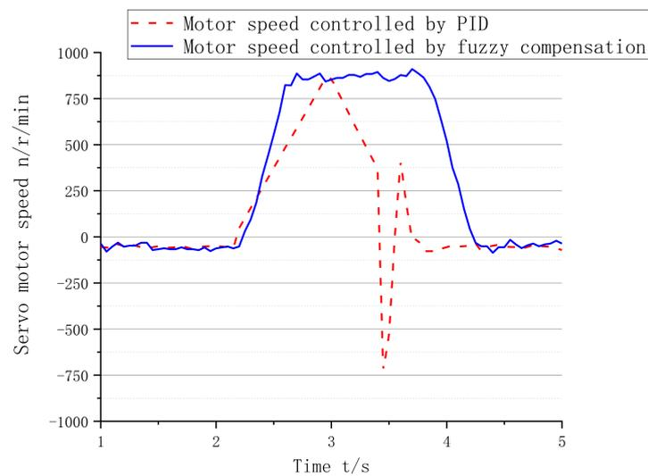
Figure 10. Speed response curve of the servo motor.
