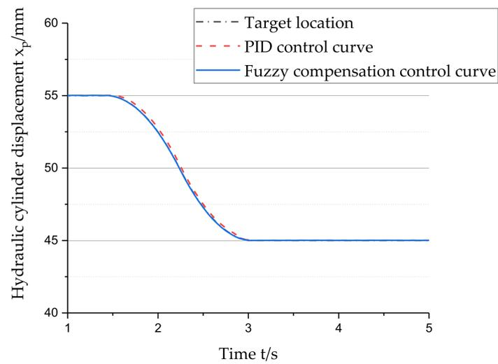
Figure 11. Response curve of the retracted position of the hydraulic cylinder.
