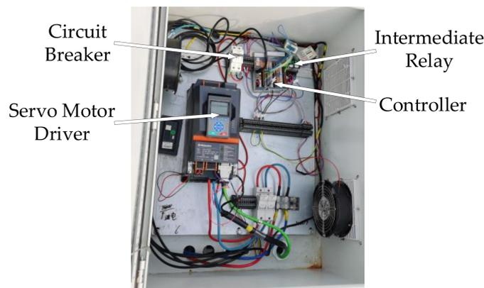
Figure 6. Electrical part of experimental platform.
