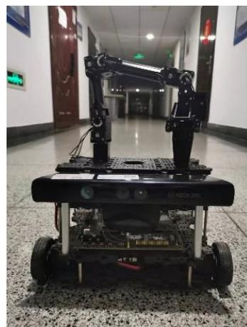
**Figure 13.** Turtlebot3 robot with Kinect camera.
