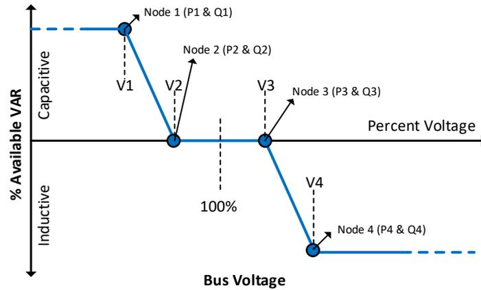
Figure 1. Array Settings of type-3 DER's Volt-VAR behavior.
