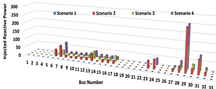
Figure 8. Reactive power injections of DERs.
