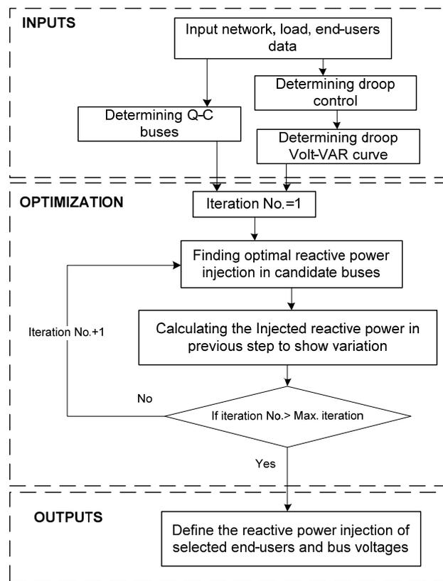
Figure 4. Schematic of the proposed algorithm.
