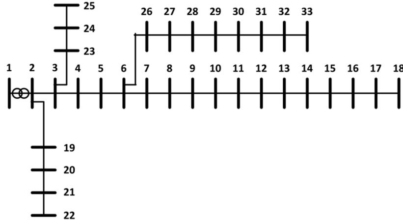
Figure 5. IEEE 33-bus standard distribution system.
