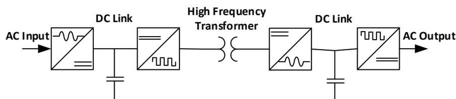
Figure 3. Power–electronic interface schematic.
