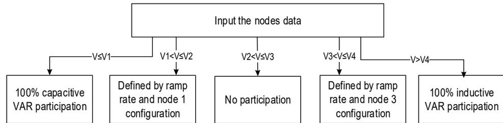
Figure 2. Desire VAR level determination algorithm.
