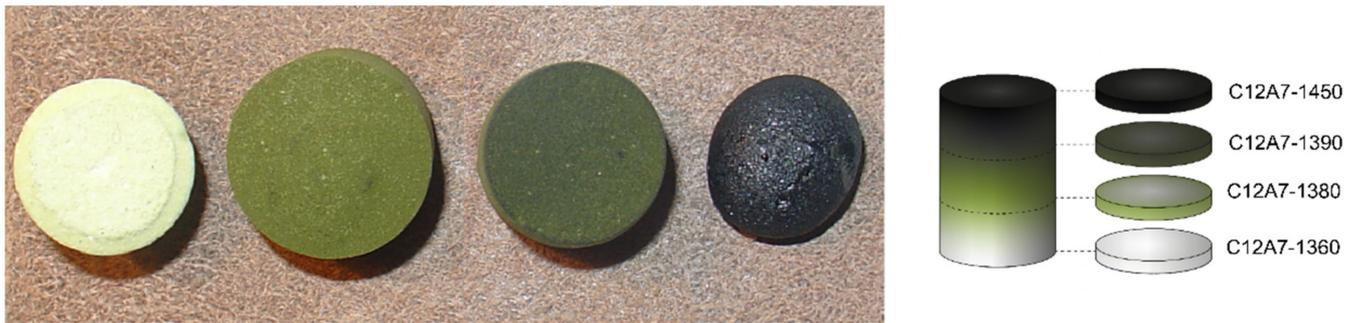
**Figure 1.** Photography and cutting scheme of samples C12A7-1360, C12A7-1380, C12A7-1390, and C12A7-1450 (from left to right).
