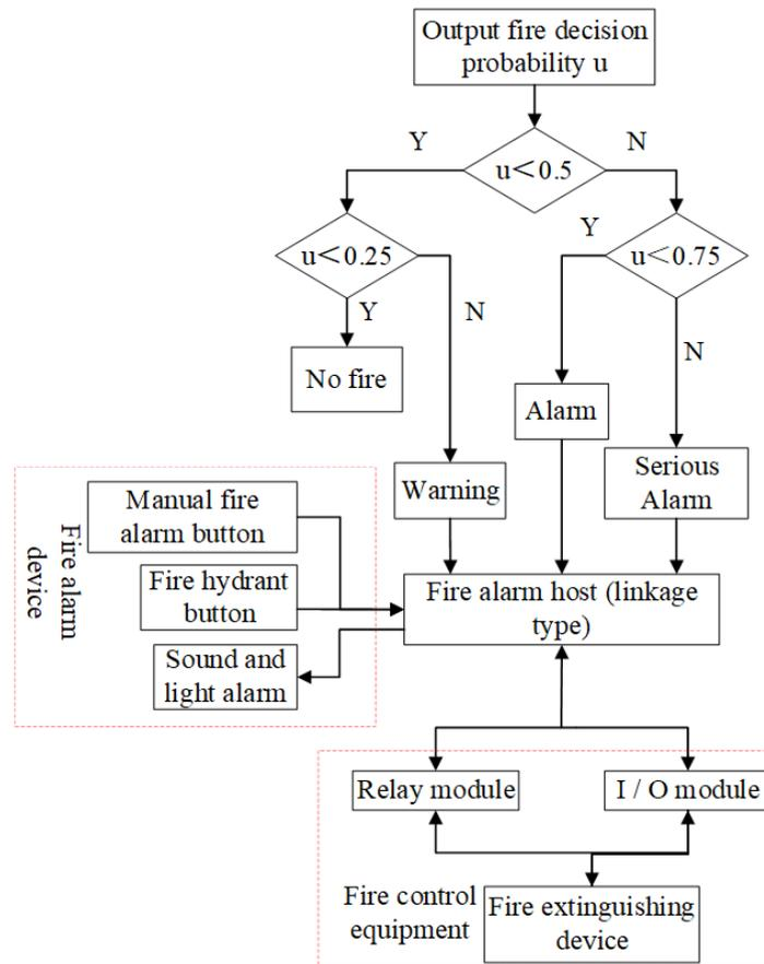
Figure 7. Flowchart of substation fire warning and fire control.
