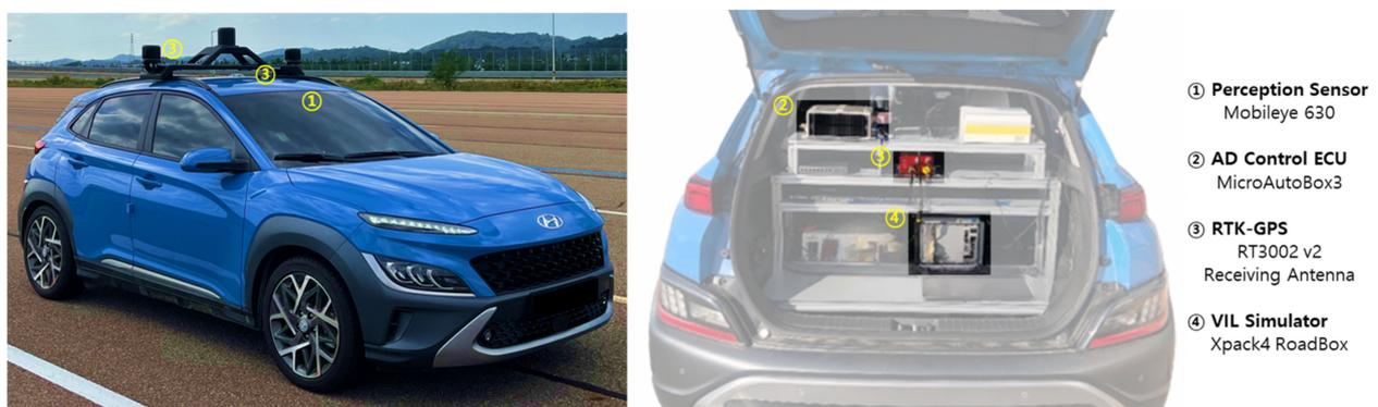
**Figure 14.** Hyundai Kona vehicle equipment components.
