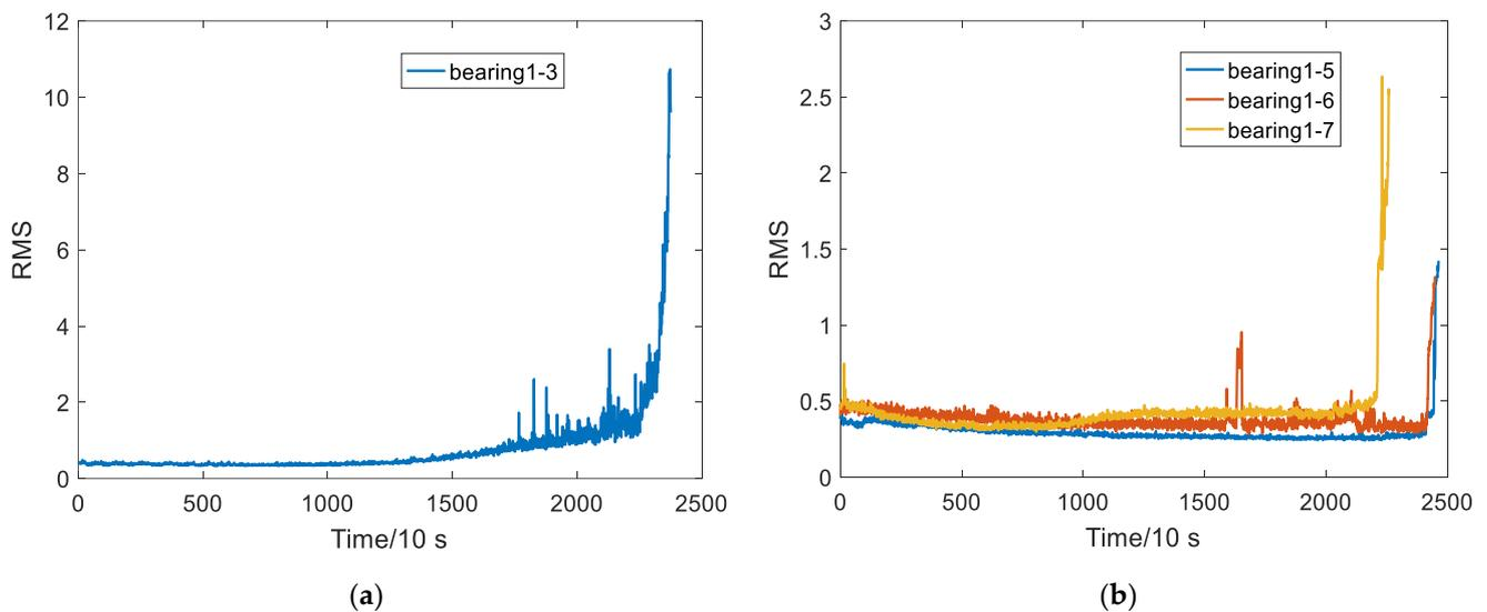
**Figure 14.** Comparison of RMSE metrics for each bearing. (a) RMS index of bearing 1–3; (b) RMS index of bearings 1–5, 1–6, and 1–7.
