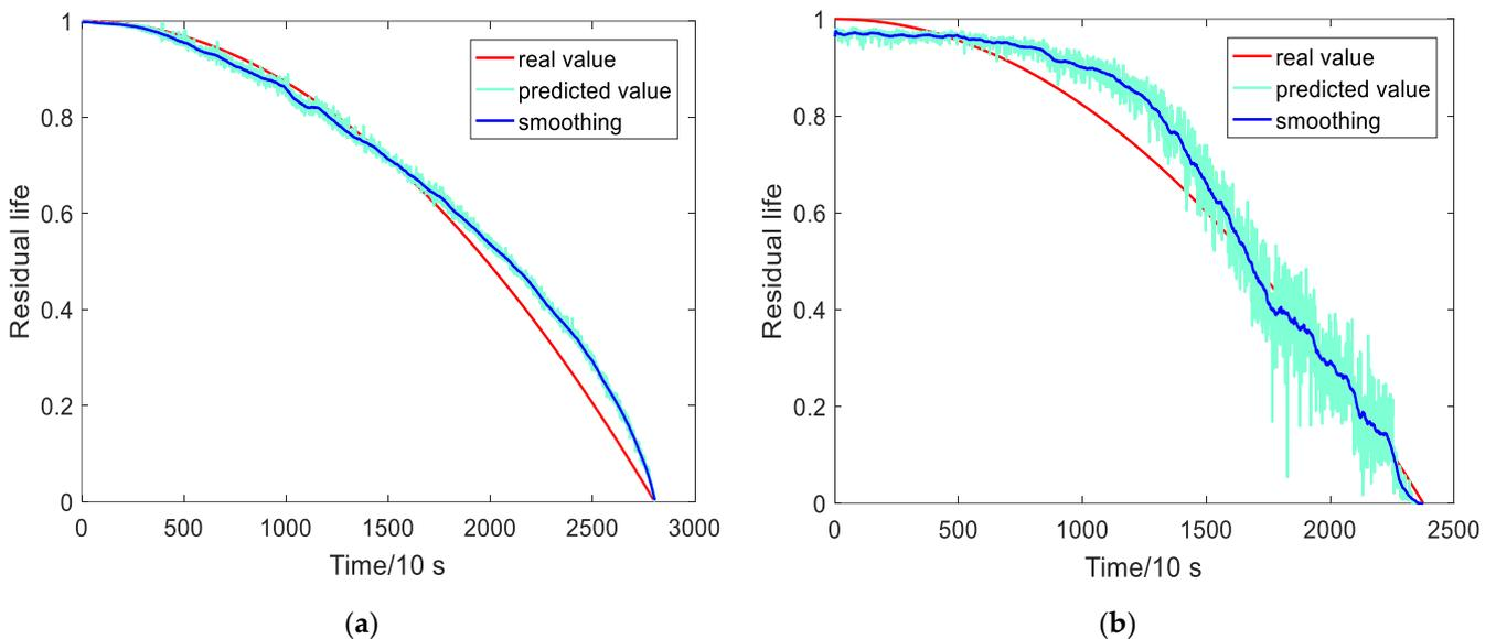
Figure 12. Prediction effect of the method in this paper on bearing 1–1 and 1–3. (a) Prediction effect on bearing 1–1; (b) Prediction effect on bearing 1–3.
