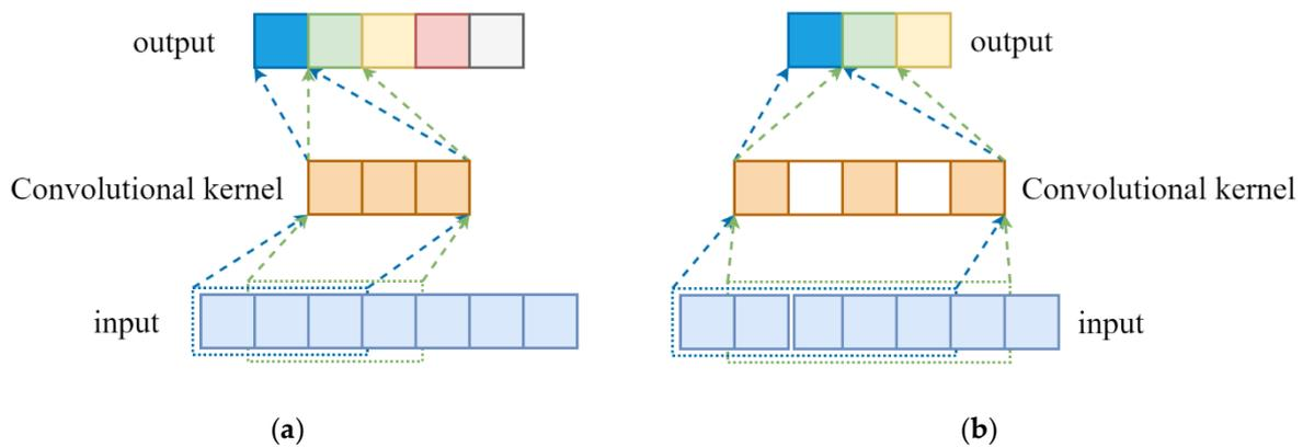
**Figure 2.** Comparison of ordinary convolution kernel and dilated convolution kernel. (a) Conventional  $1 \times 3$  convolution kernel; (b) Dilated convolution  $1 \times 3$ , dilation rate is 2.
