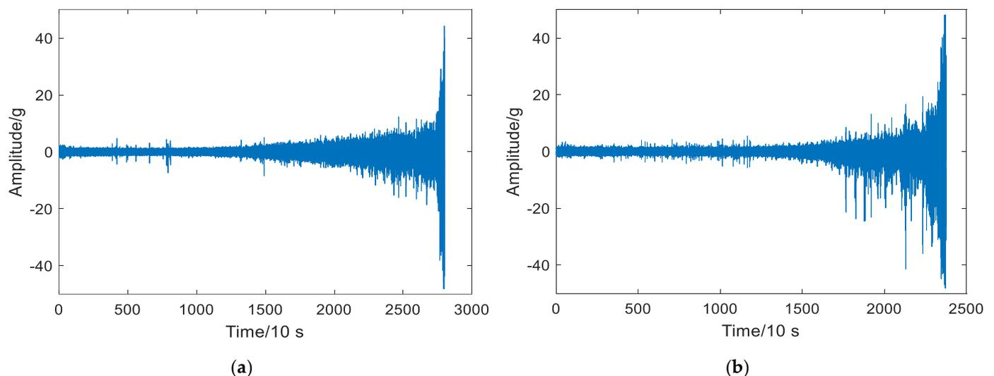
**Figure 7.** Time domain signal waveforms of bearing 1-1 and 1-3. (a) Time domain waveform of bearing 1-1; (b) Time domain waveform of bearing 1-3.
