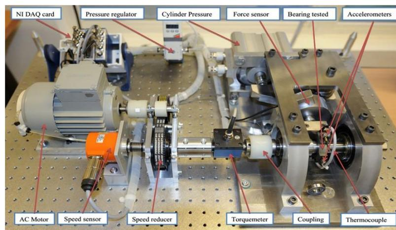
**Figure 6.** PRONOSTIA experimental platform.
