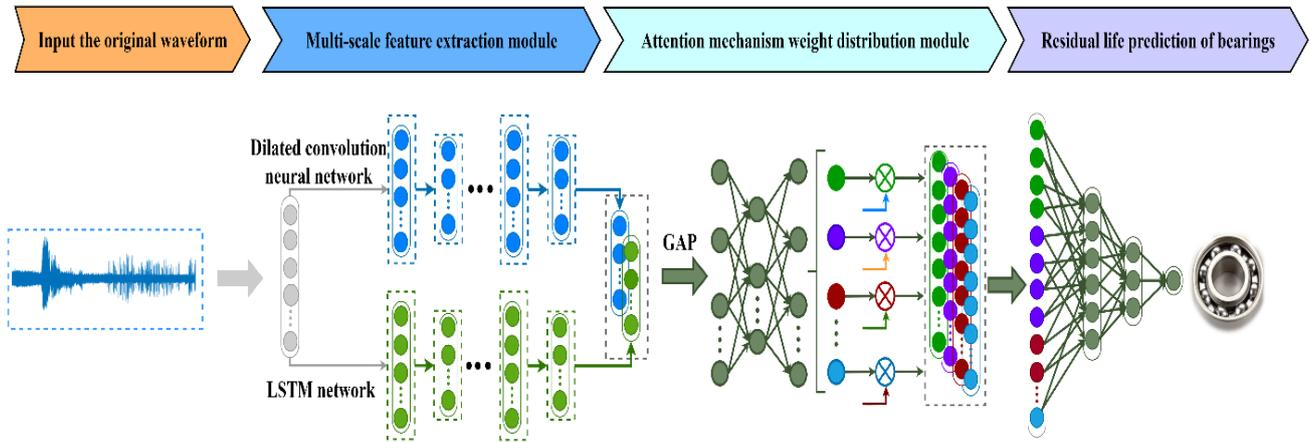
**Figure 4.** Network model of rolling bearing remaining life prediction method based on multi-scale feature extraction and attention mechanism.
