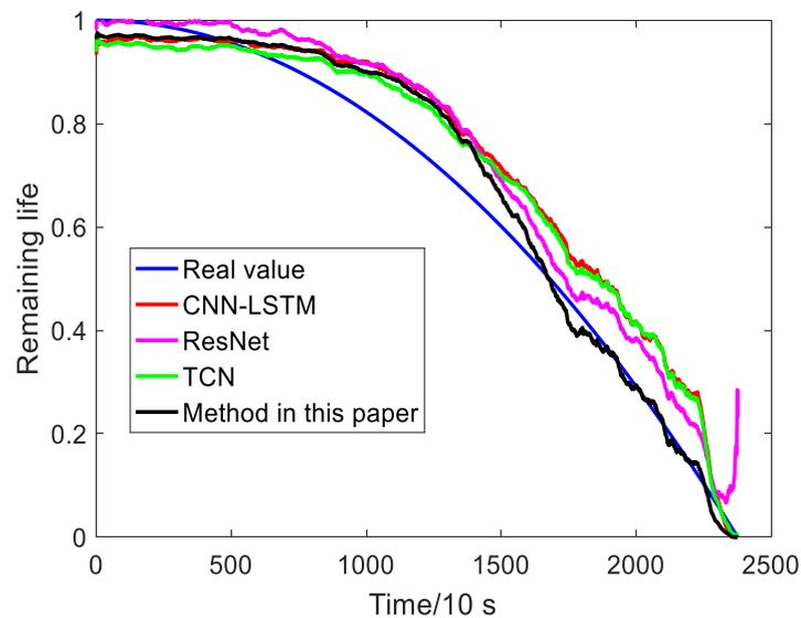
Figure 13. RUL prediction results of each method on test bearing 1–3.
