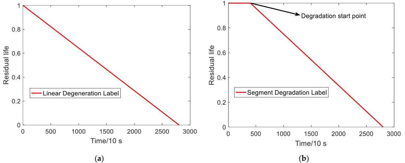
**Figure 8.** Two commonly used degradation labels. (a) Linear degeneration label; (b) Segment degradation label.
