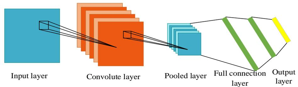
Figure 1. Basic structure of CNN.
