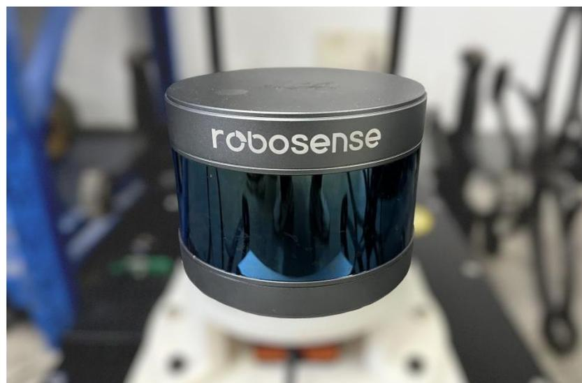
**Figure 12.** RS-LiDAR-16 used in our test.
