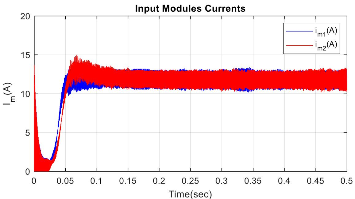
Figure 12. Experimental waveforms of the module input currents in the converter.
