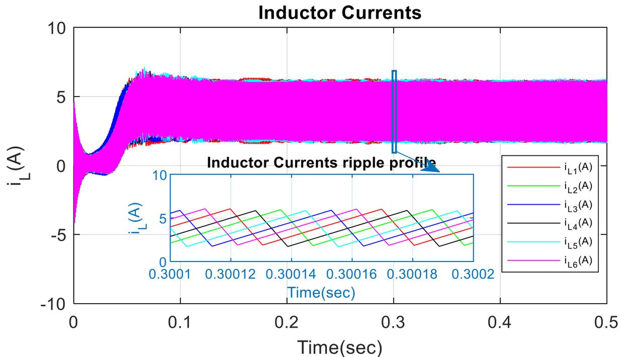
Figure 11. Experimental waveforms of the inductor currents in six phases.
