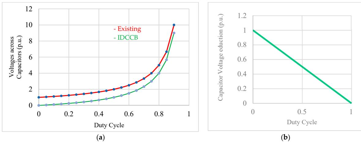
**Figure 5.** Capacitor voltage profiles (a) p.u. capacitor voltages [16] and (b) Reduced p.u. stresses on capacitors in existing and proposed IDCCB (the base value is the input voltage).
