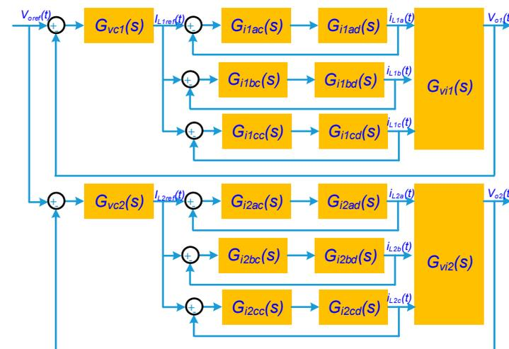
Figure 8. Control diagram of the implemented controller.
