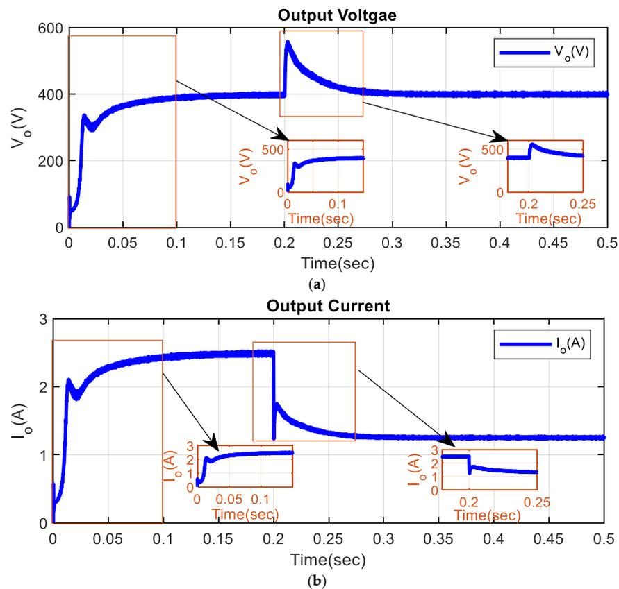
Figure 15. Load parameters during load change from 1000 W to 500 W.
