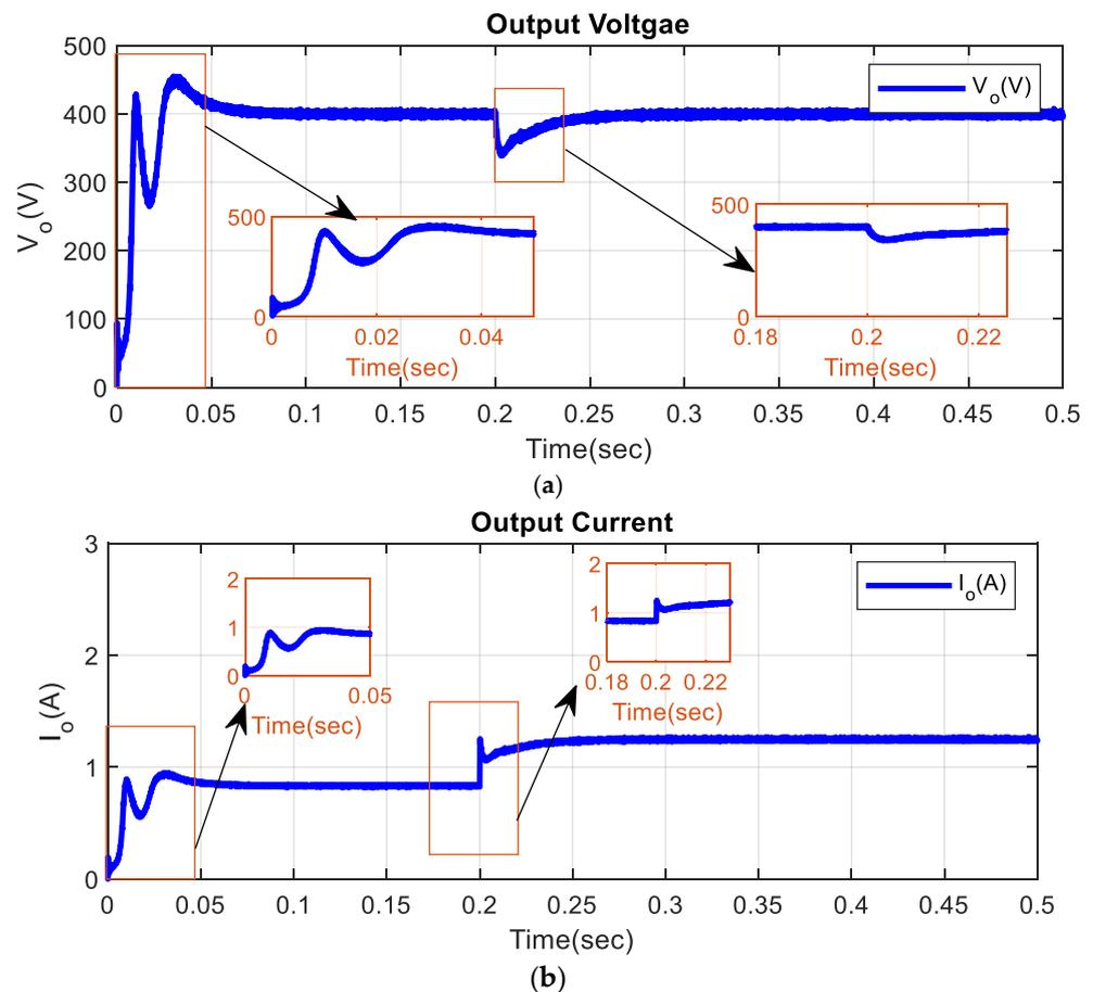
**Figure 16.** Load parameters during load change from 500 W to 1000 W.
