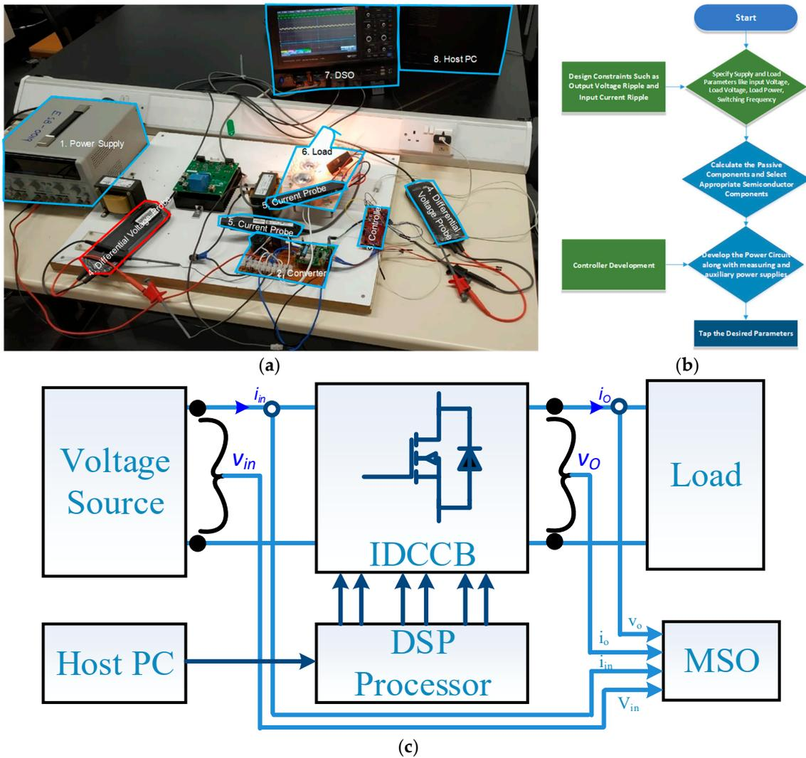
**Figure 10.** (a) Experimental setup: (1) power supply; (2) IDCCB converter; (3) DSP controller; (4) voltage probes; (5) current probes; (7) digital storage oscilloscope; (8) host PC. (b) Design guidelines flowchart for the IDCCB and (c) block diagram of the hardware setup.
