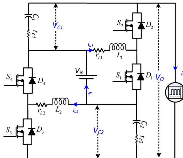
Figure 2. Interleaved differential capacitor clamped boost converter.
