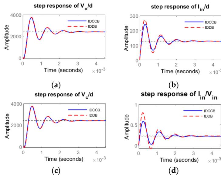
**Figure 6.** Set of probable equilibrium points: (a) output voltage-to-duty ratio ( $V_o/d$ ); (b) input current-to-duty ratio ( $I_{in}/d$ ); (c) capacitor voltage-to-duty ratio ( $V_c/d$ ); (d) input current-to-input voltage ( $I_{in}/V_{in}$ ) transfer functions of the IDDB and IDCCB.
