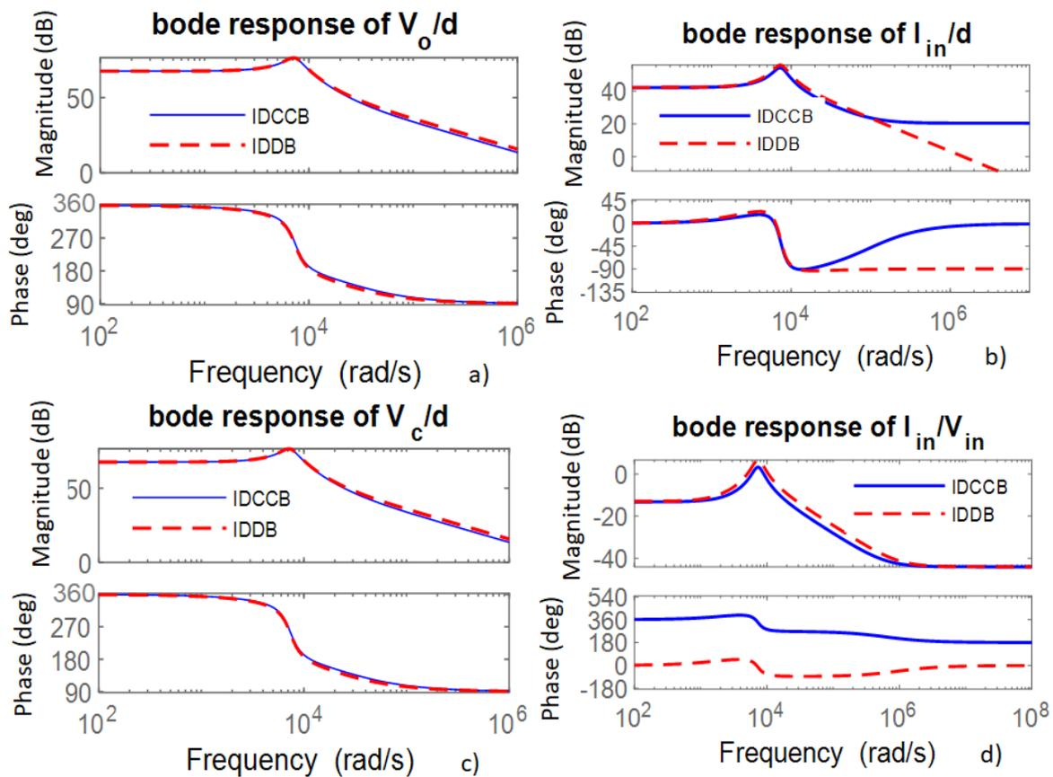
**Figure 9.** Bode plots: (a) output voltage-to-duty ratio ( $V_o/d$ ); (b) input current-to-duty ratio ( $I_{in}/d$ ); (c) capacitor voltage-to-duty ratio ( $V_c/d$ ); (d) input current-to-input voltage ( $I_{in}/V_{in}$ ) transfer functions for the IDCCB.
