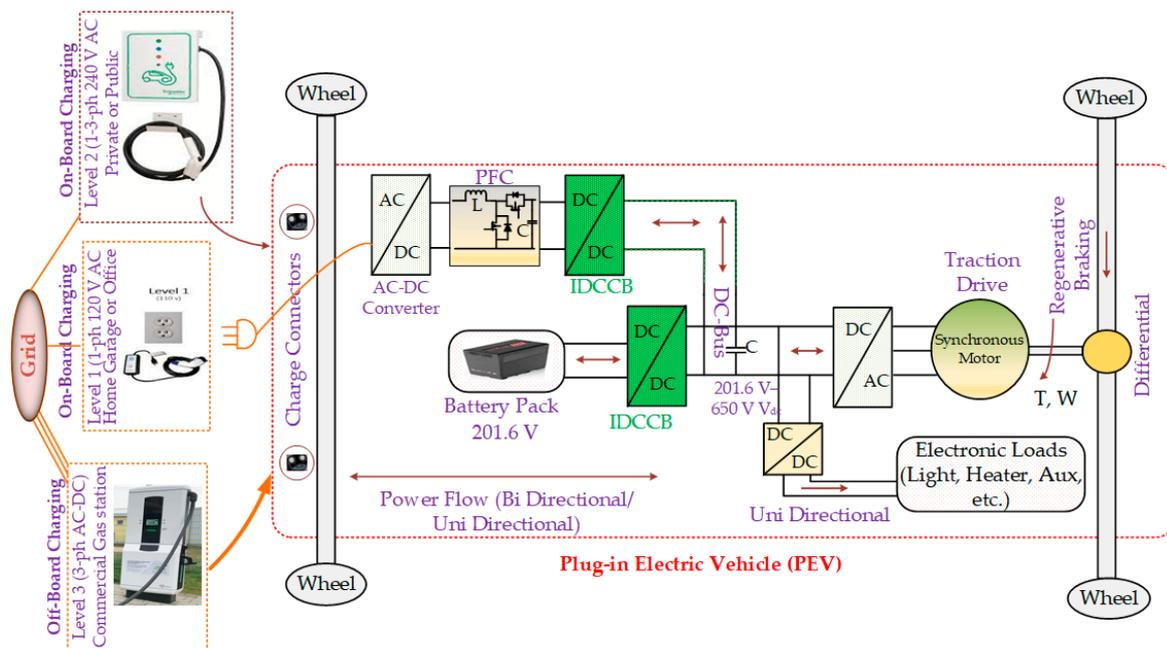
Figure 1. Architecture of a plug-in electric vehicle.
