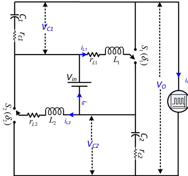
Figure 3. Interleaved capacitor clamped boost converter.
