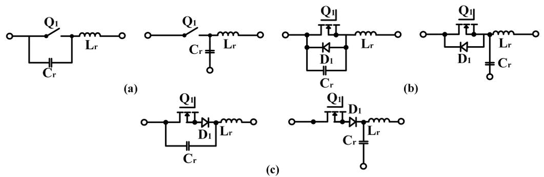
**Figure 3.** Voltage mode resonant switches: (a) m-type, l-type configurations, (b) half-wave mode, and (c) full-wave mode.
