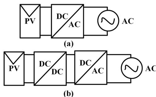
**Figure 1.** Types of PV inverters: (a) single stage, (b) multi stage [5].
