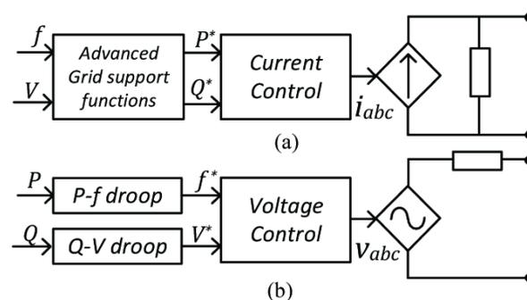
**Figure 20.** Inverter controllers: (a) grid-following control with grid support functions; and (b) grid-forming droop control [122].
