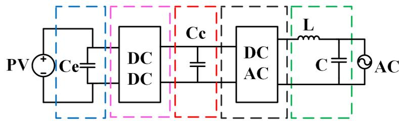
**Figure 2.** Conventional scheme used for multi-stage PV-connected applications.
