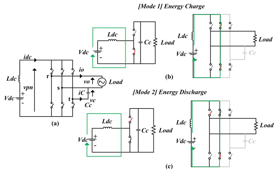
Figure 17. Topologies: (a) structure of the single-phase current source inverter with power decoupling function, (b) boost technique of conventional circuit, (c) boost technique of the presented circuit.
