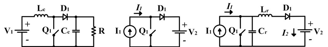
**Figure 4.** Boost converter : (left) common structure, (middle) steady-state equivalent circuit, and (right) ZVS quasi-resonant converter.
