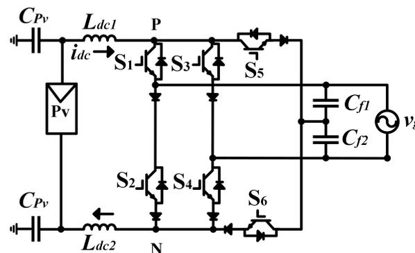
Figure 19. CSI with AC-side clamping [135].
