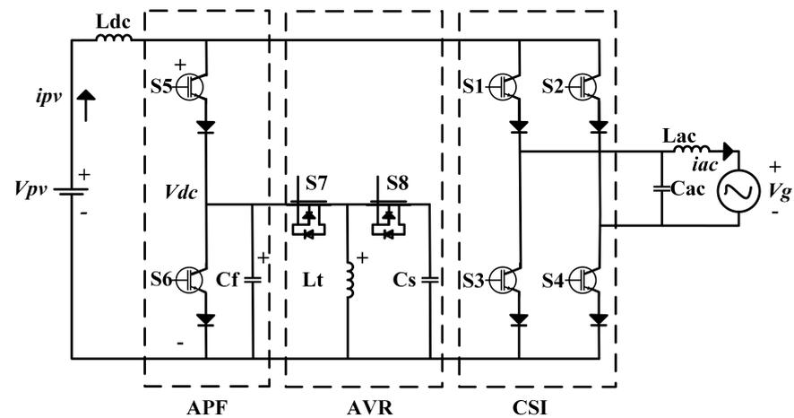
Figure 16. Power decoupling circuit for CSI.
