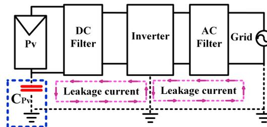
Figure 18. Simplified common-mode leakage current.
