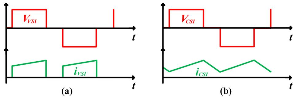
**Figure 11.** Voltage and current representation over one switching period at the entrance of the inverter: (a) VSI and (b) CSI.
