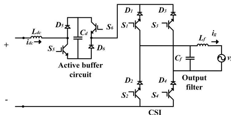
**Figure 14.** Single-phase current source converter.
