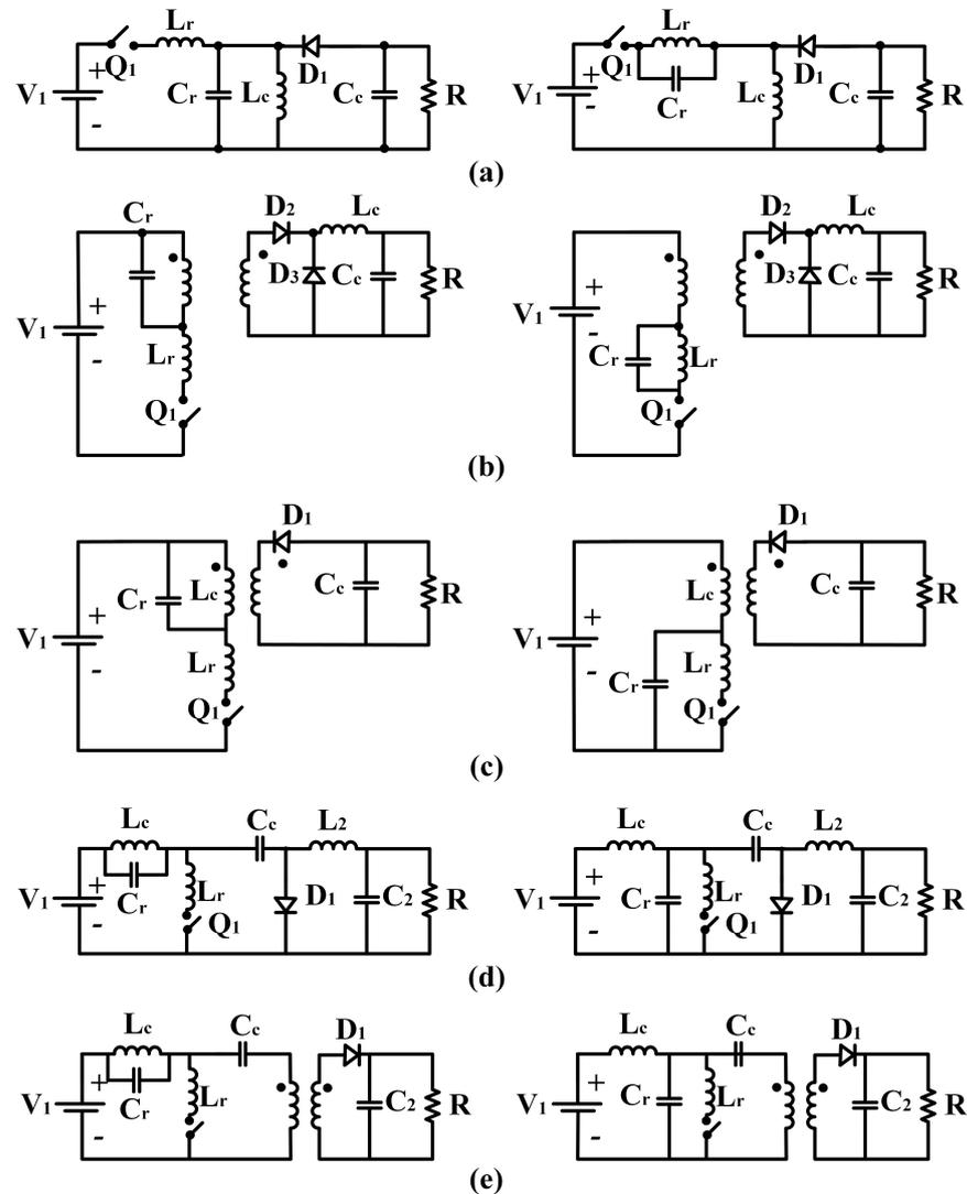
Figure 7. Quasi-resonant topologies: (a) buck-boost, (b) forward, (c) flyback, (d) Ćuk, and (e) SEPIC.
