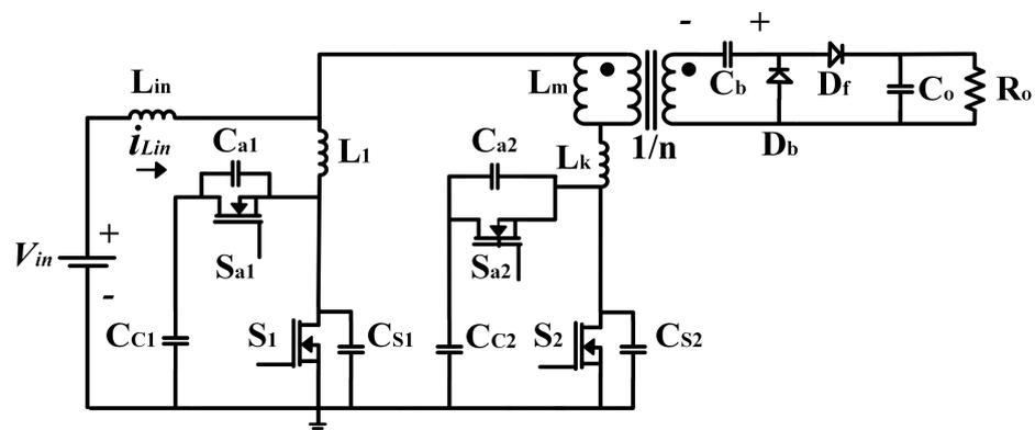
Figure 10. High step-up current-fed converter.
