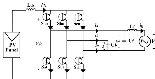
**Figure 15.** CSI with six voltage bidirectional switches.
