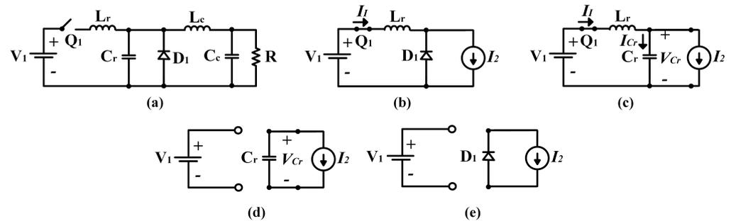
**Figure 6.** Topology and operation modes: (a) quasi-resonant buck converter, (b) charging of  $L_r$ , (c) resonant mode, (d) discharging of  $L_r$ , and (e) freewheeling mode.
