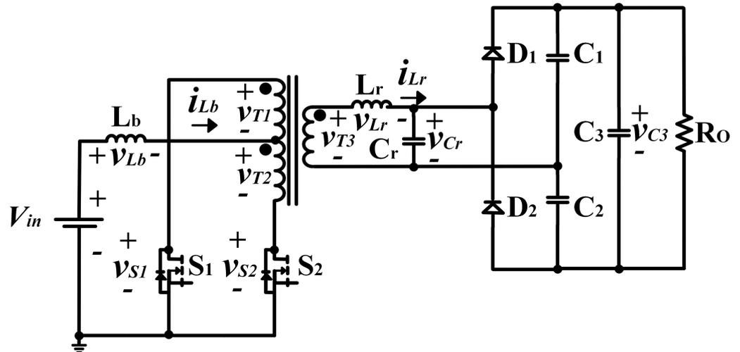
Figure 9. Push-pull converter.
