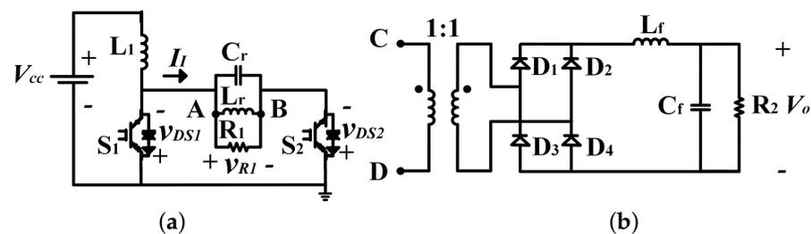
Figure 8. Resonant converter. (a) CSPRC, (b) adding transformer and rectifier.
