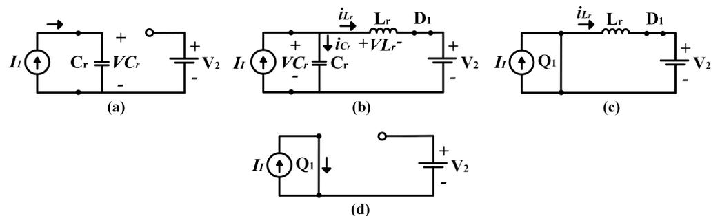
**Figure 5.** Operation modes: (a) charging of  $C_r$ , (b) resonant mode, (c) discharging of  $C_r$ , and (d) freewheeling mode.
