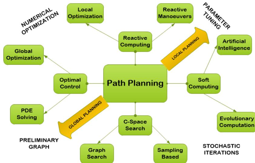
Figure 1. Schematic showing different path planning methods.
