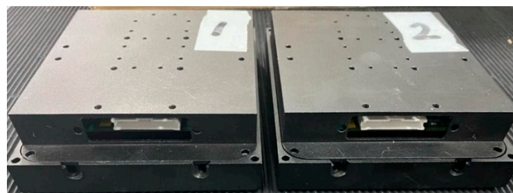
Figure 6. Dummy EDFA units for the preliminary radiation tests.
