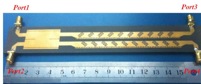
Figure 14. Photograph of the fabricated antenna.
