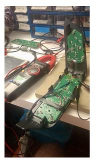
Figure 5. PCB with sensors based on a mutual-capacitance design assembled on a plastic part.
