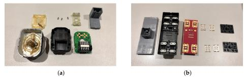
**Figure 16.** Example of the number of components and complexity of (**a**) side mirror's and (**b**) windows' control buttons
