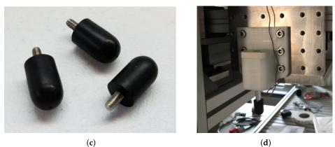
**Figure 9.** The figure depicts the testing environment specifically designed and developed from scratch to validate the touch-based prototype. In (**a**) the structure of the CNC is shown. (**b**) Depicts the CNC controller board with digital inputs. (**c**) Illustrates the the "finger" probes that emulate a human touch. The gripper in (**d**) was custom-designed and printed using 3D printing technology to allow attachment the probe to the moving part of the CNC strucutre.
