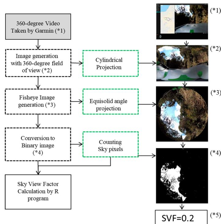
**Figure 1.** Flowchart of sky view factor (SVF) calculation.
