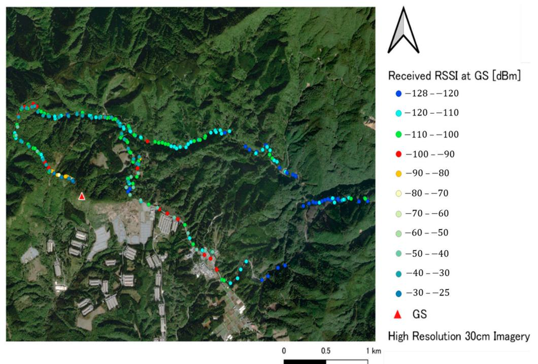
Figure 3. Experimental measured data on a map.
