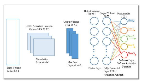
Figure 11. Fully connected Layer [8].
