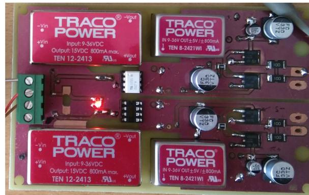
Figure 14. The driver PCB.
