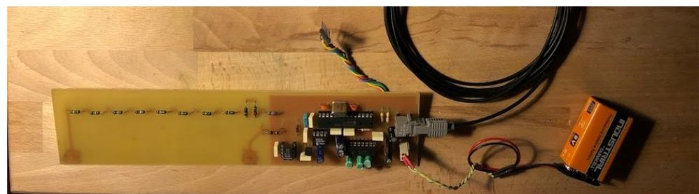
Figure 15. The high voltage measuring board PCB.
