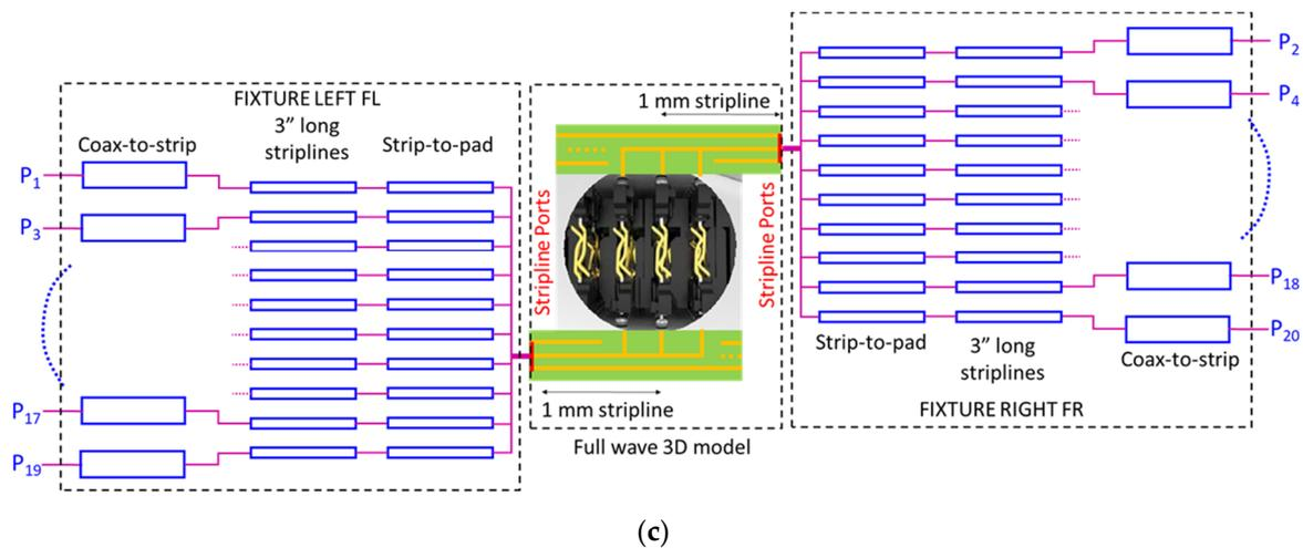
**Figure 3.** (a) Overview of the full de-embedding setup, (b) details of the FL and FR fixtures, (c) complete fixtures from the original multiport model.
