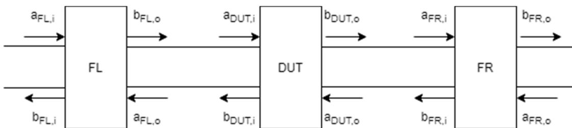
Figure 2. System of three 2-port S-parameter networks to be cascaded.
