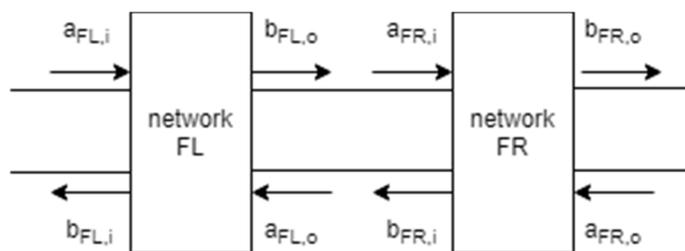
**Figure 1.** Cascade of two 2-port S-parameter networks: “FL” stands for left feature network and “FR” stands for right feature network.
