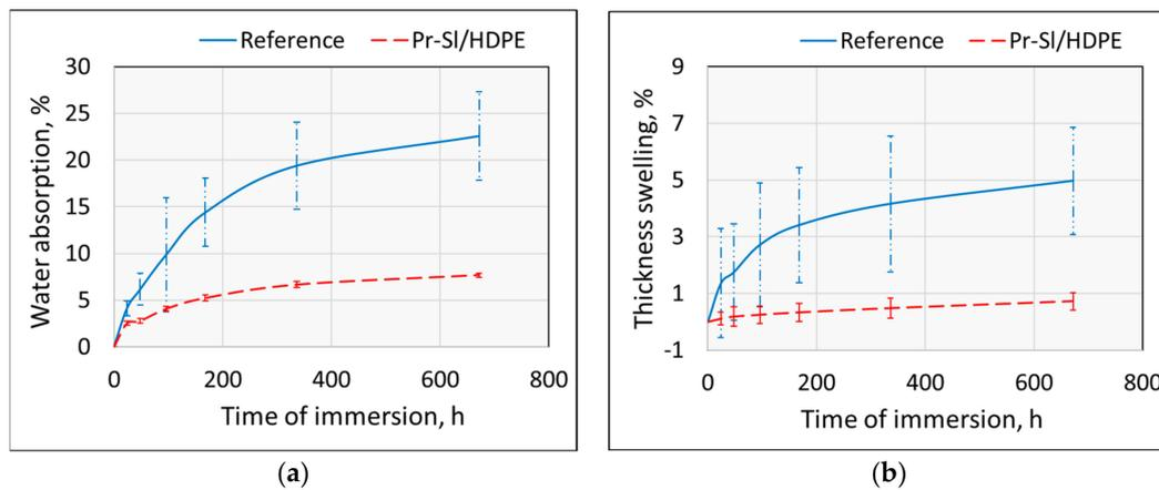
**Figure 3.** Water absorption (a) and thickness swelling (b) of the studied materials. The uniform line represents the reference material and the discontinuous line represents the Pr-SI/HDPE material. The results consist of average values, with error bars describing the standard deviations.
