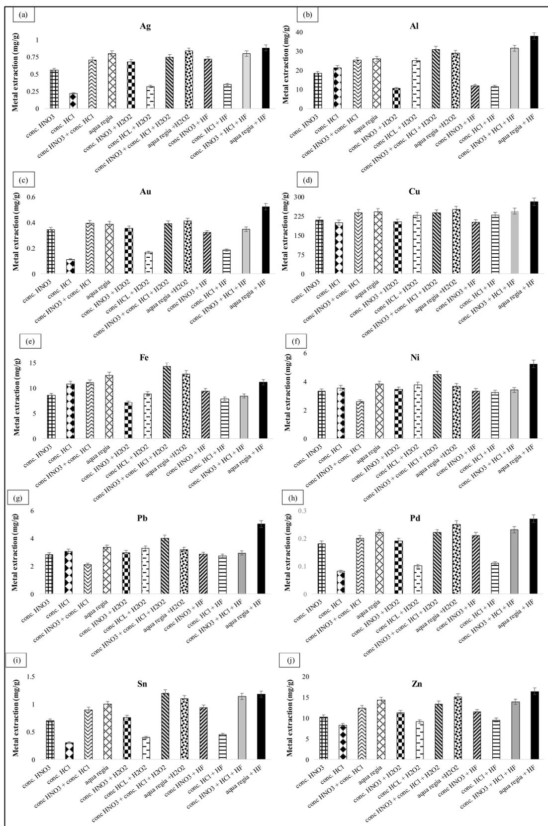
**Figure 3.** Dissolution of metals (a) Silver (Ag); (b) Aluminum (Al); (c) Gold (Au); (d) Copper (Cu); (e) Iron (Fe); (f) Nickel (Ni); (g) Lead (Pb); (h) Palladium (Pd); (i) Tin (Sn); (j) Zinc (Zn) using different acids ( $n = 3$ ).
