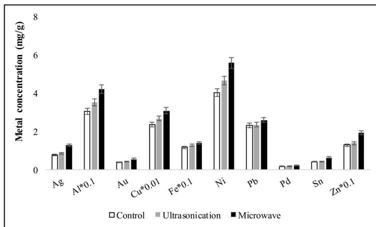
**Figure 6.** Effect of different driving forces on metal recovery from TES-AMM samples using the US EPA SW 846 Method 3050b, ( $n = 3$ ). (For instance, the Cu\*0.01 value of 3 denotes a Cu concentration of 300 mg/g.)
