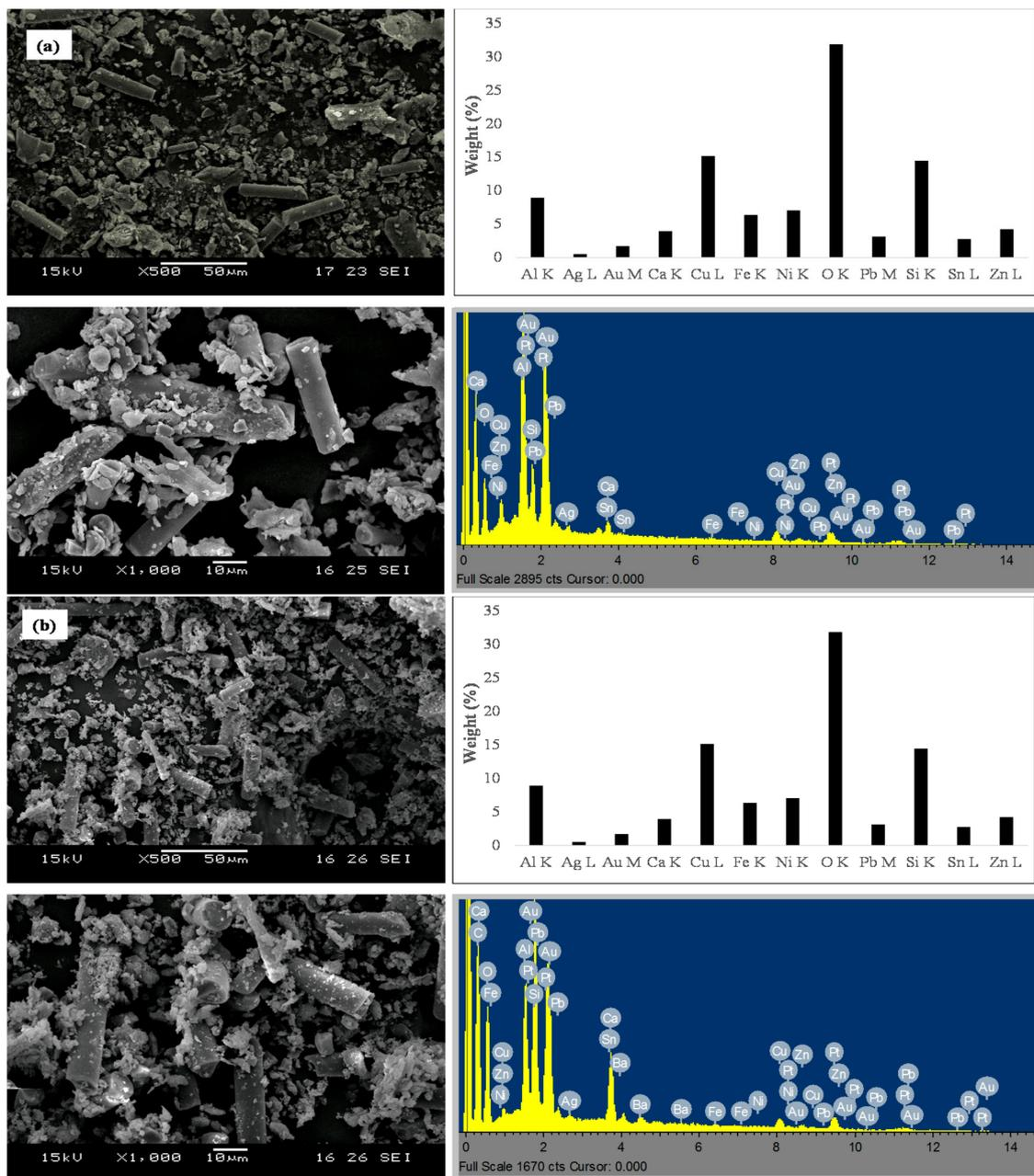
**Figure 1.** SEM-EDX micrographs of untreated ESM samples obtained from (a) TES-AMM and (b) CRR.
