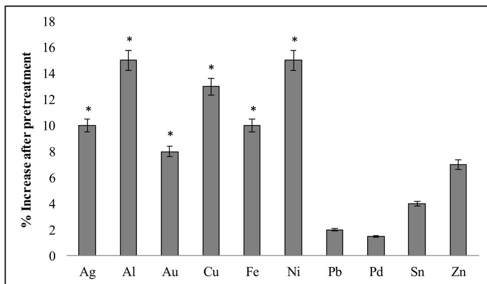
**Figure 5.** Impact of pretreatment on recovery of metal from ESM using ASTM D6357-11 Method, ( $n = 3$ ,  $p < 0.05$ , one-way ANOVA, “\*” indicates significant effect of pretreatment).
