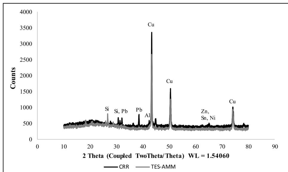
**Figure 2.** XRD analysis of untreated ESM samples obtained from CRR and TES-AMM.
