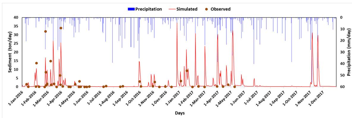
Figure 6. Time series graph comparison of observed sediment loads with simulated sediment loads over the period of 2016–2017 of the Wigle Creek watershed.
