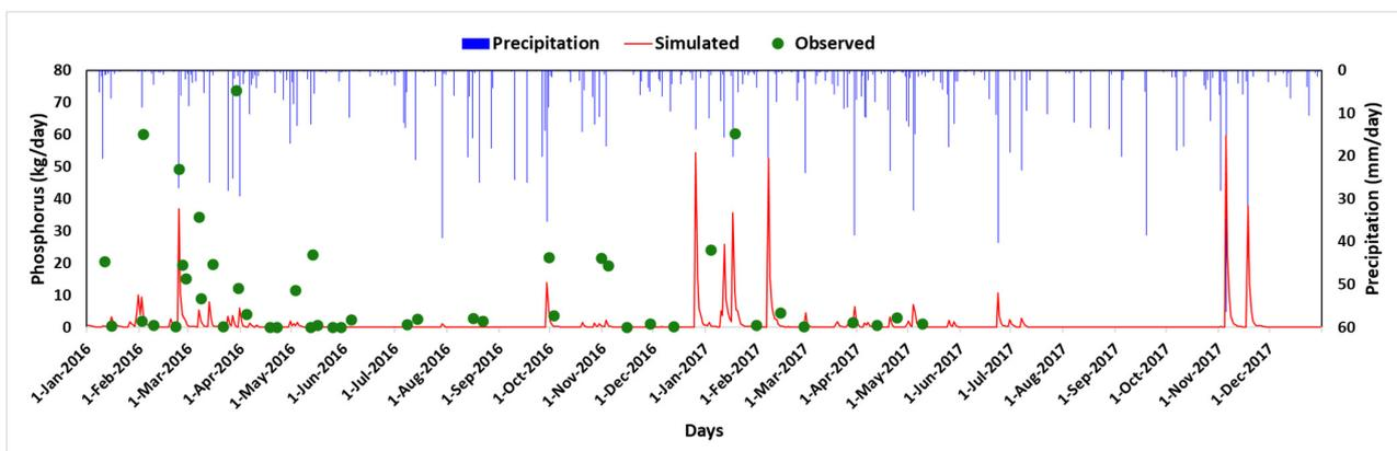
**Figure 8.** Time series graph comparison of observed phosphorus loads with simulated phosphorus loads during the period of 2016–2017.
