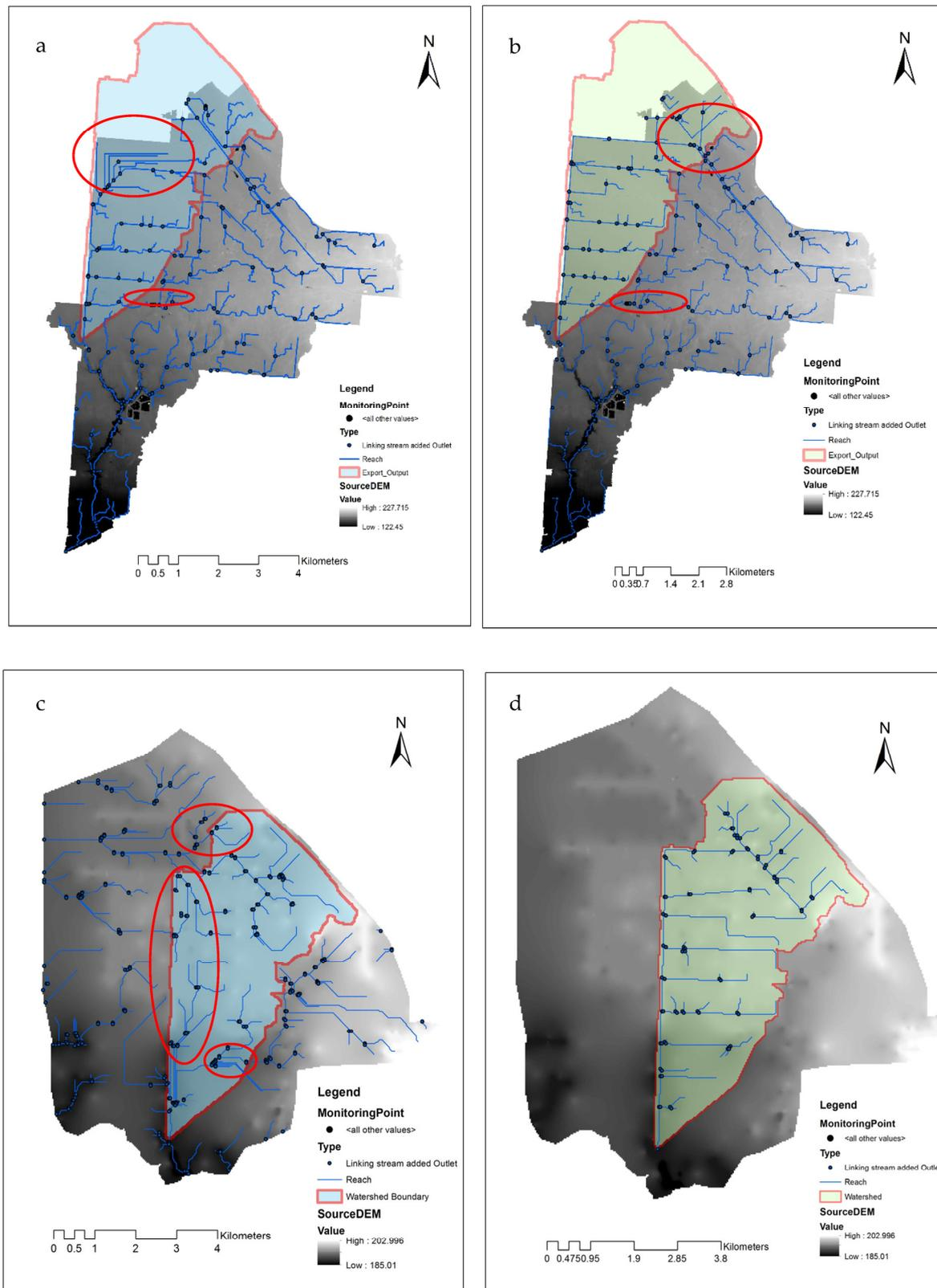
**Figure 3.** Stream-framework delineation for the Wigle Creek watershed: (a) stream network generated with the 0.5 m × 0.5 m Hydro-Enforced DEM, (b) modified burn-in stream network based on the 0.5 m × 0.5 m Hydro-Enforced DEM, (c) stream network generated with the 30 m × 30 m DEM, and (d) modified burn-in stream network on the 30 m × 30 m DEM.
