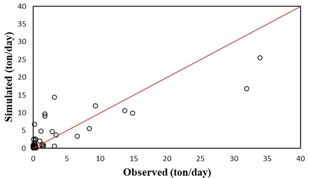
**Figure 7.** Scatter plot between observed and simulated sediment loads of the Wagle Creek watershed during the period of 2016–2017.
