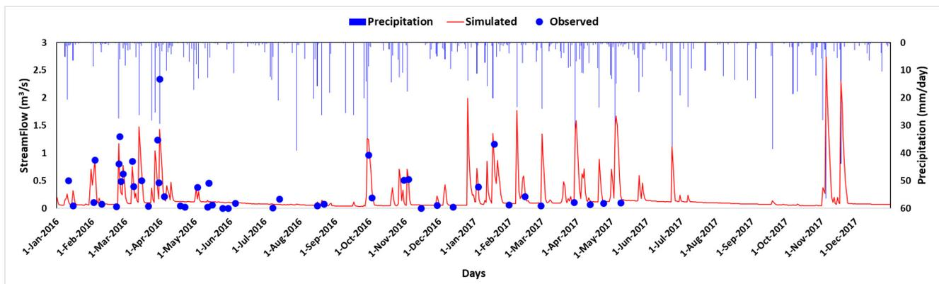
**Figure 4.** Time series comparison graph of observed with simulated streamflow loads of the Wigle Creek watershed over the period of 2016–2017.
