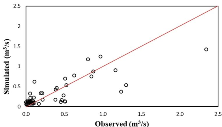
Figure 5. Scatter plot between observed and simulated streamflow datasets of the Wigle Creek watershed during the period of 2016–2017.
