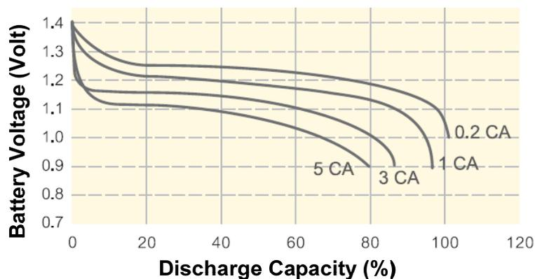
In our circuit, battery voltage is detected during this period to accurately estimate the energy stored in the battery. Depending on the detected  $V_{bat}$ , the power-performance of the integrated electronic circuits and operation duty cycle of the wireless transceiver are reconfigured to guarantee autonomous
