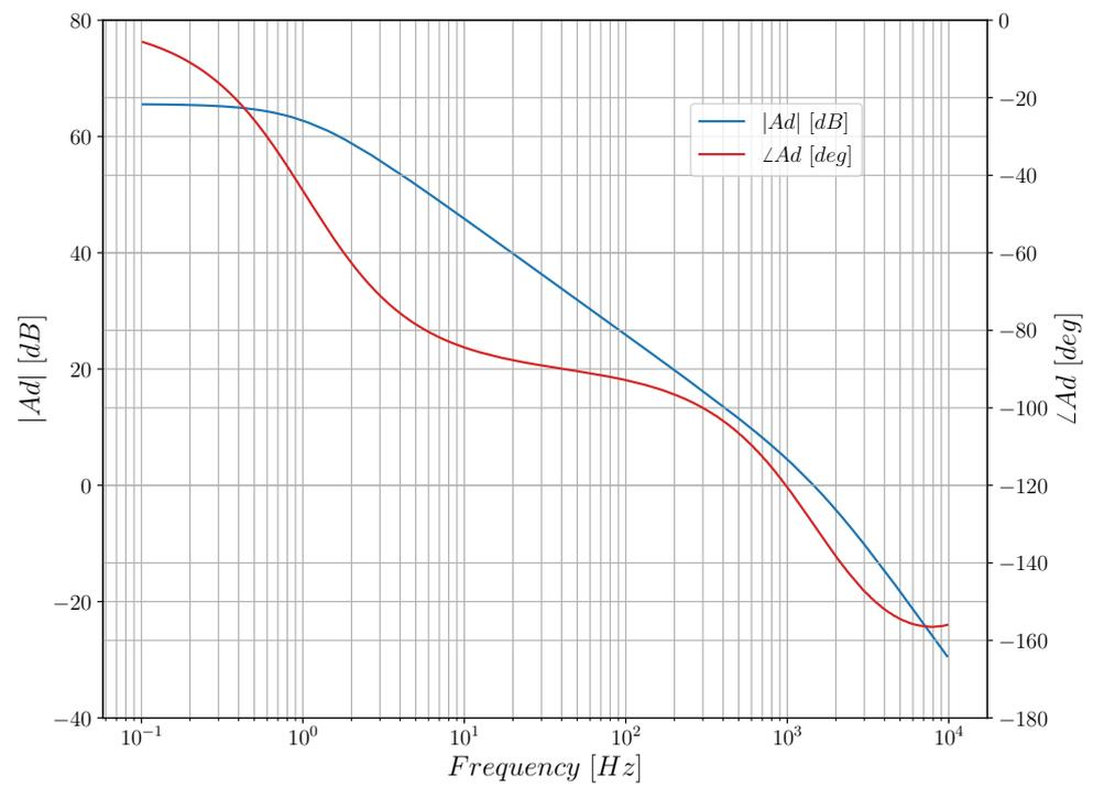
Figure 4. Differential-mode transfer function.
