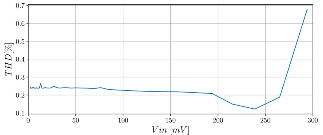
Figure 8. Total harmonic distortion vs. input peak-to-peak voltage.
