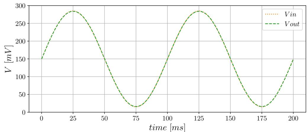
Figure 9. Response of the proposed OTA to a 10 Hz 270 mVpp sinusoidal input signal.
