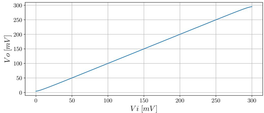
**Figure 10.** Input–output DC characteristic in a non-inverting buffer configuration.
