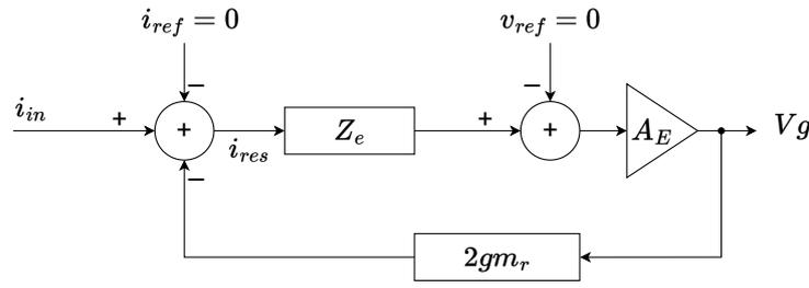
**Figure 2.** Block scheme of the replica bias loop.
