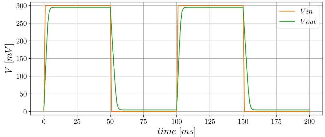
Figure 7. Step response in unity-gain closed-loop configuration.
