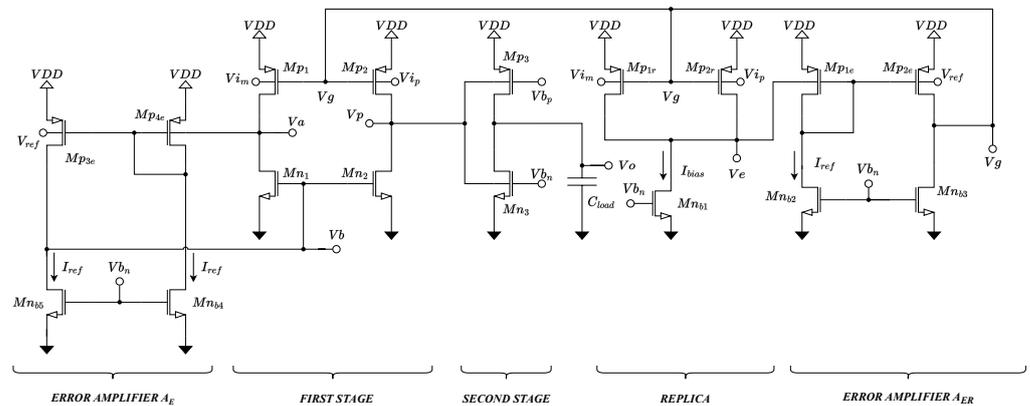
Figure 1. Proposed two-stage OTA architecture with enhanced current mirror and replica bias.
