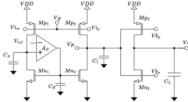
Figure 3. Schematic of the amplifier for small-signal analysis.
