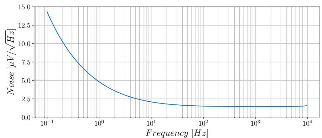
Figure 6. Input-referred noise spectrum.
