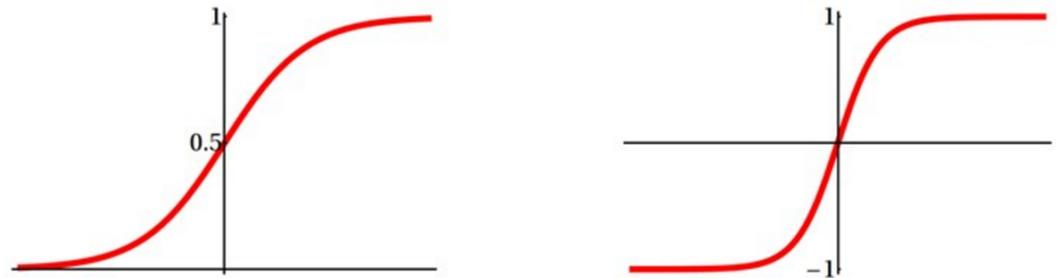
**Figure 18.** Logistic function (left) and hyperbolic tangent function (right).
