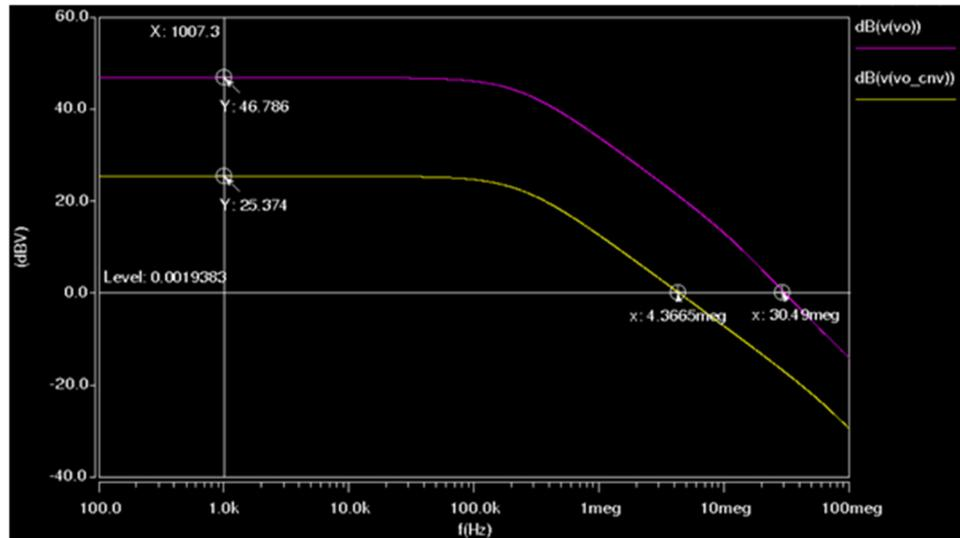
Figure 2. AC open-loop response in 22 nm.
