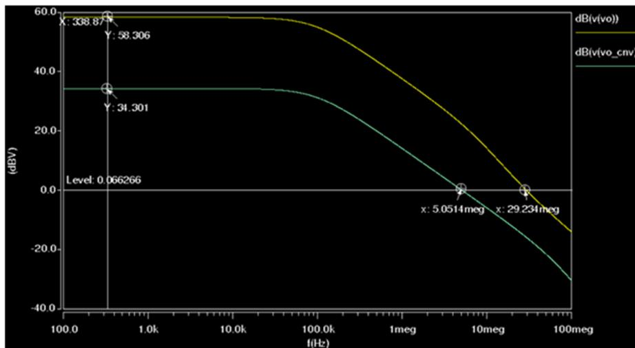
Figure 5. AC open-loop response in 180 nm.
