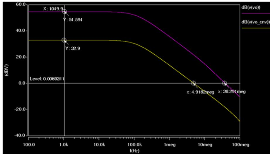
Figure 4. AC open-loop response in 90 nm.
