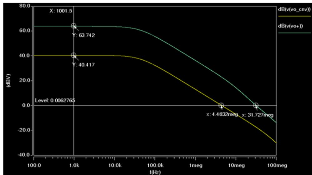
Figure 3. AC open-loop response in 45 nm.
