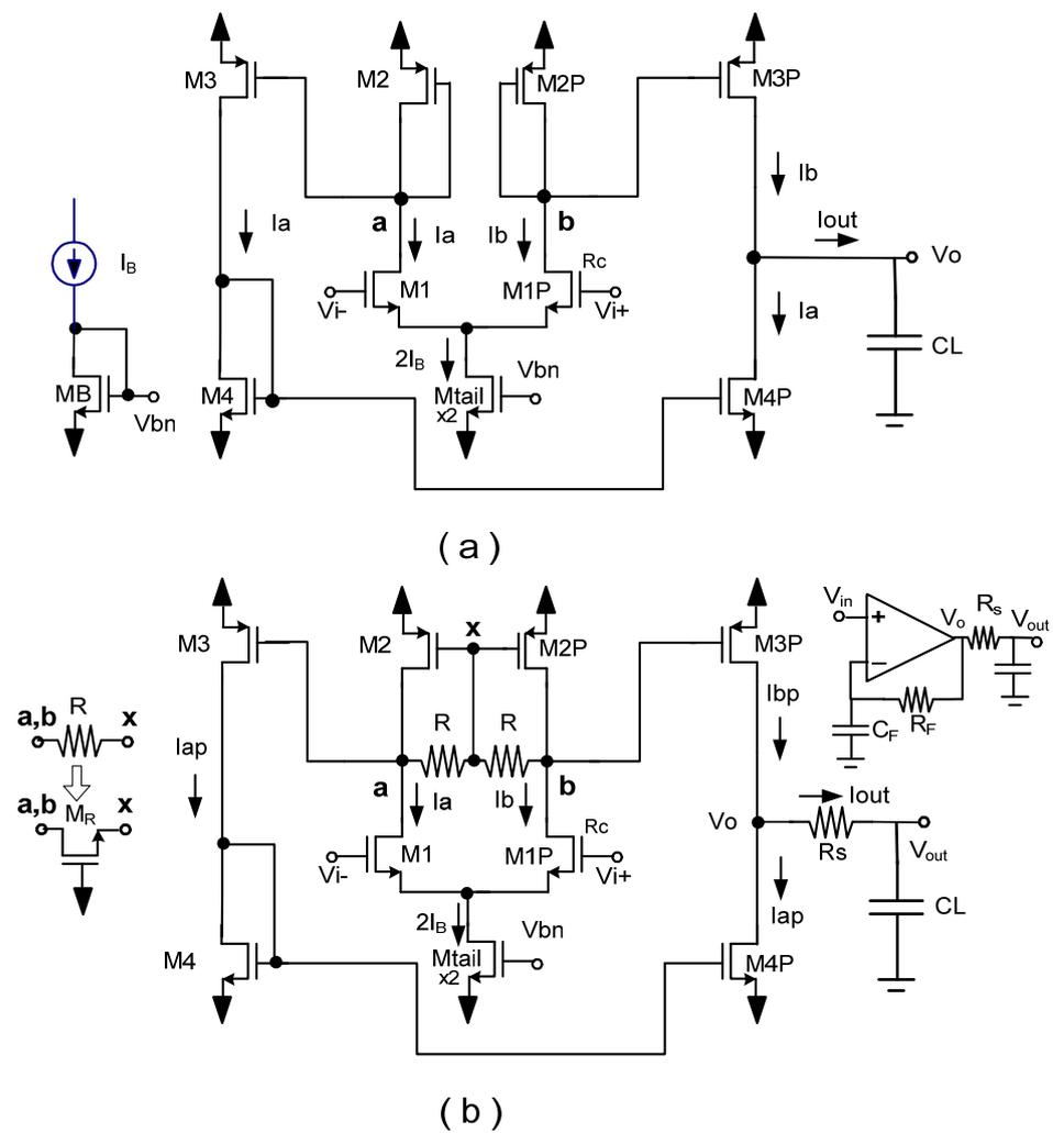
**Figure 1.** (a) Conventional one-stage op-amp without cascoding transistors. (b) One-stage op-amp with resistive local common mode feedback.
