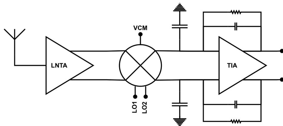
**Figure 2.** Cascaded receiver diagram.
