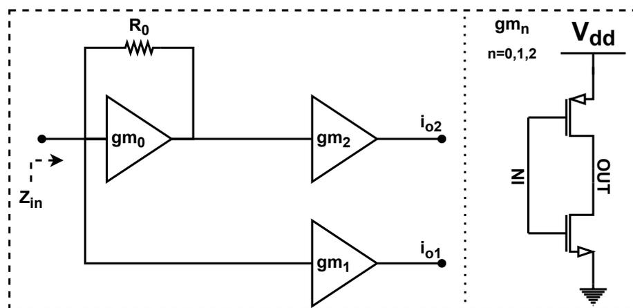
**Figure 3.** LNTA circuit diagram.
