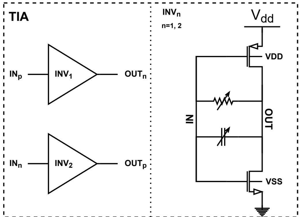
Figure 5. TIA circuit diagram.
