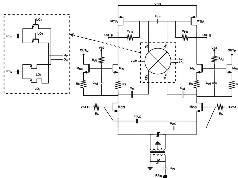
Figure 4. Stacked receiver circuit diagram.
