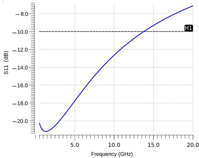
Figure 6. The cascaded received input matching (S11) performance versus RF.
