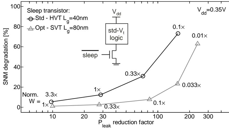
Therefore, a sleep-mode leakage reduction technique is preferred. Amongst them, power gating relies on the addition of a high- $V_t$  sleep transistor to cut off the leakage path in sleep mode. The effective  $E_{cycle}$  can thus be expressed as [24]:
