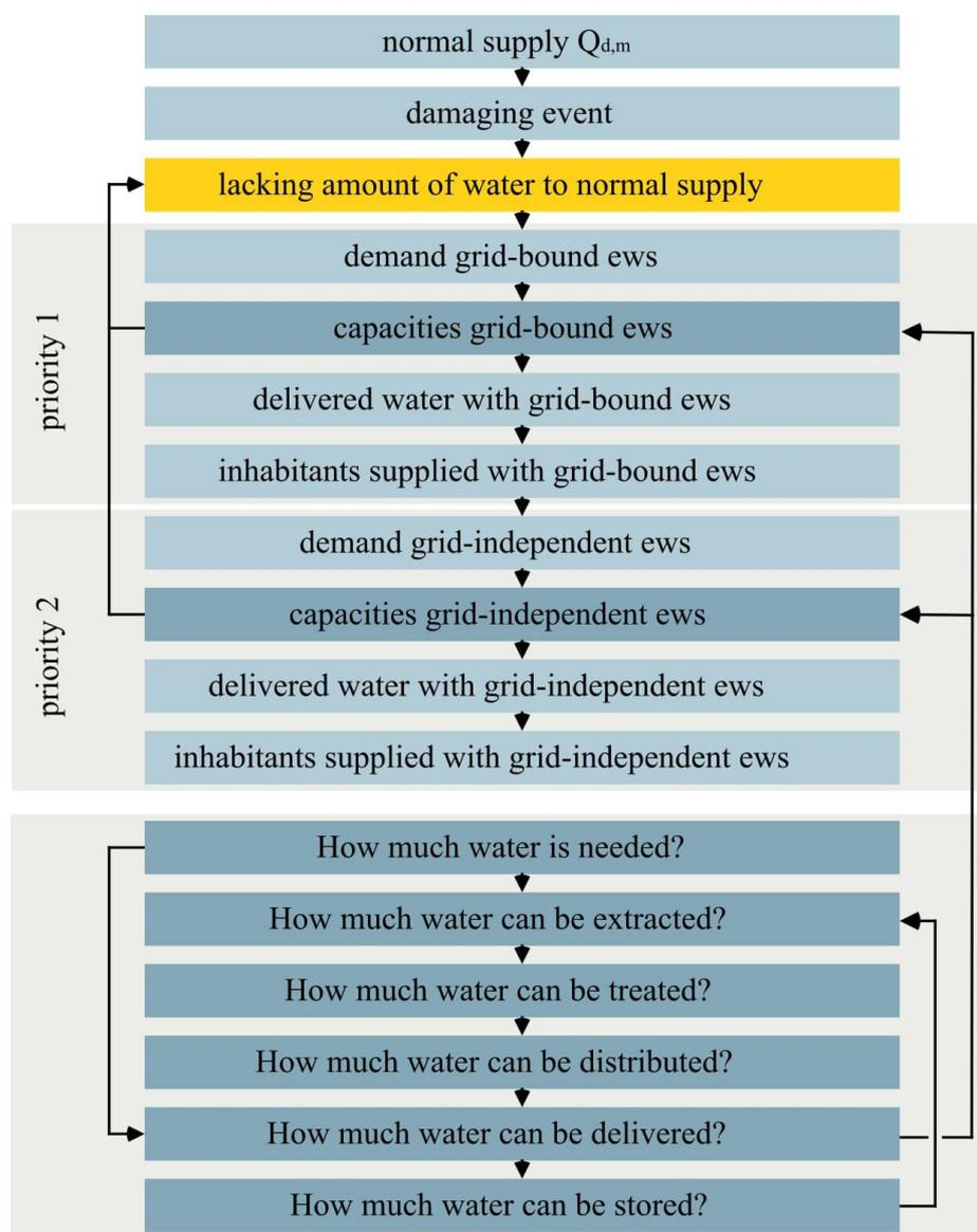
Figure 4. Structure of the system dynamics (SD) model.
