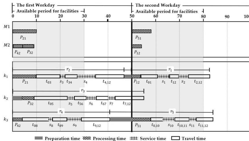
**Figure 2.** Gantt chart of loading scheme and trip scheduling (NV = 3).
