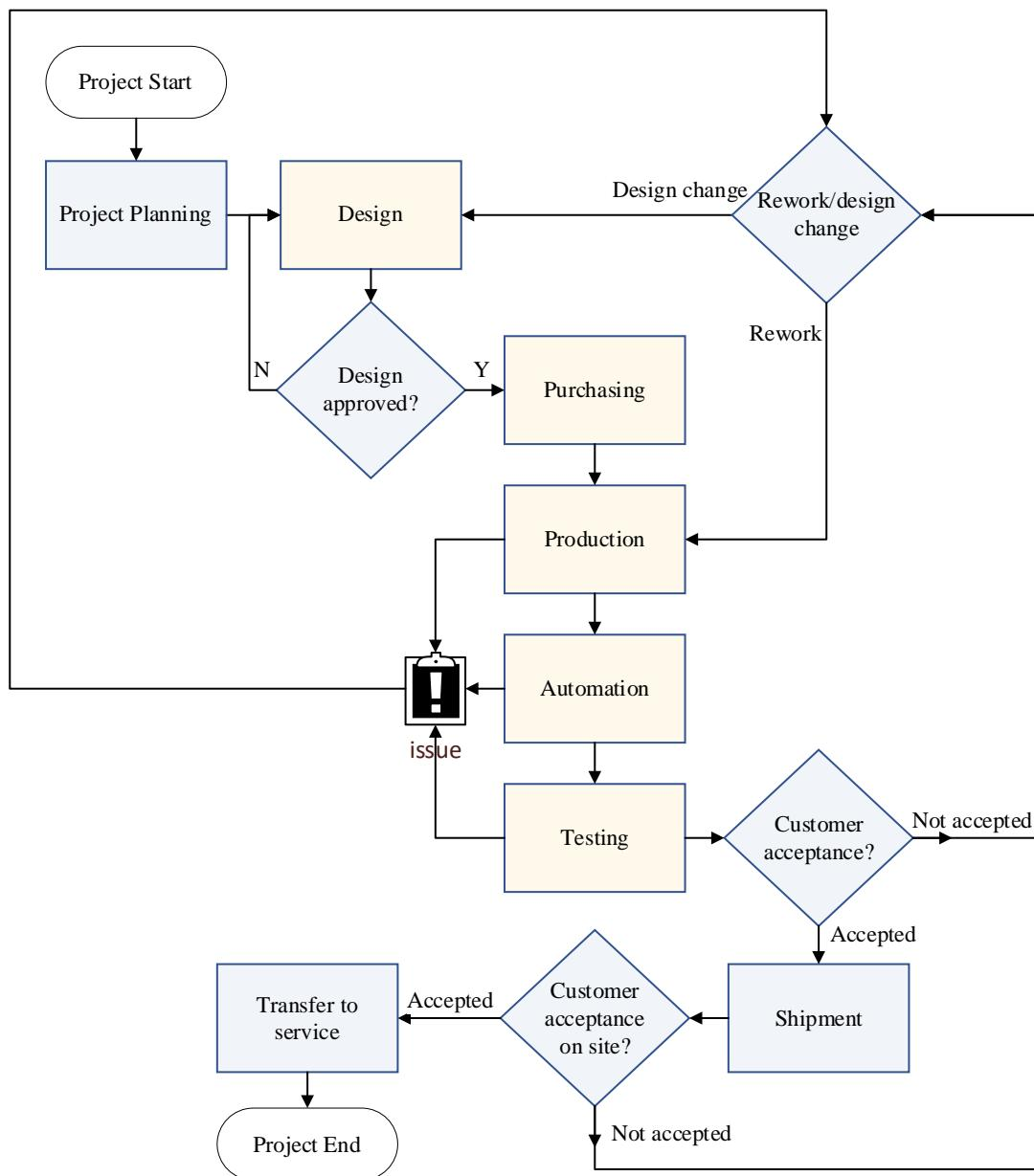
**Figure 1.** Phases for a machine development project.
