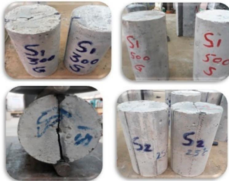
**Figure 7.** RPC samples at different burning temperatures and steel fiber volume fraction percentage after splitting tensile strength test.
