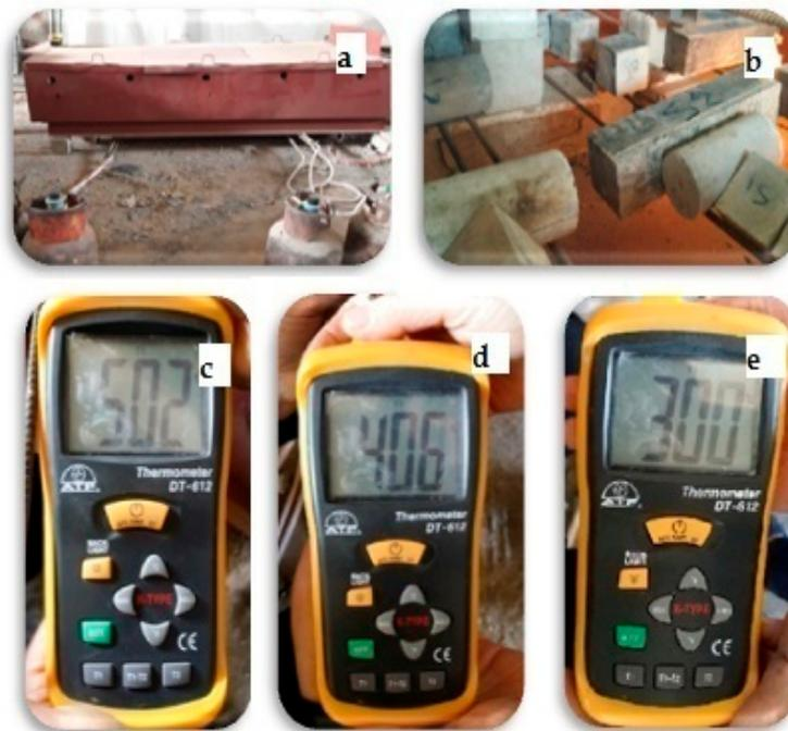
**Figure 1.** Burning process: (a) Burning furnace setup; (b) Samples inside the furnace; (c) Thermocouple device at 500 °C; (d) Thermocouple device at 400 °C; (e) Thermocouple device at 300 °C.
