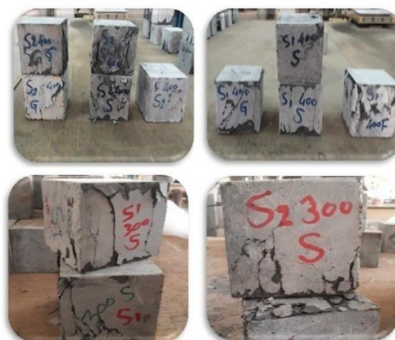
**Figure 3.** RPC samples at different burning temperatures and steel fiber volume fraction percentage after compressive strength test.
