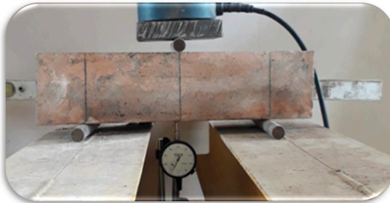
Figure 11. A sample of deflection determination for 1.0%  $V_f$  at 400 °C with gradual-cooling method.
