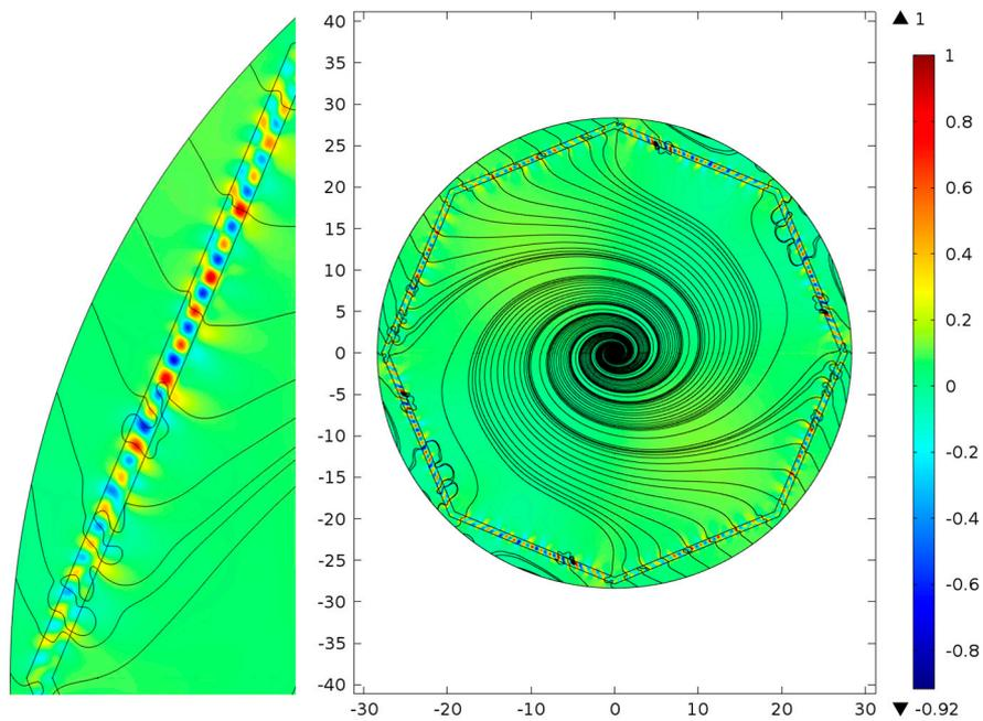
**Figure 3.** Distribution of the transverse Poynting vector component projection on the radius vector direction in the silica glass octagon waveguide microstructure cross section. The streamlines for the transverse component of Poynting vector (black lines).
