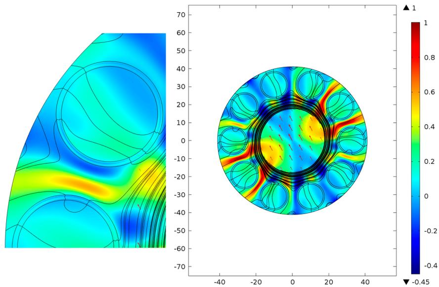
**Figure 6.** Distribution of the transverse Poynting vector component projection on the radius vector direction in the cross section of a silica glass NCHCF with ten non-contacting cladding capillaries. The streamlines for the transverse component of Poynting vector (black lines).
