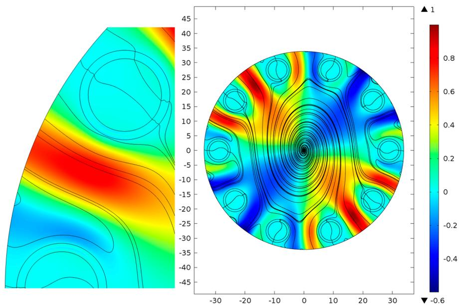
**Figure 7.** Distribution of the transverse Poynting vector component projection on the radius vector direction in the cross section of a silica glass NCHCF with ten non-contacting cladding capillaries. The streamlines for the transverse component of Poynting vector (black lines).
