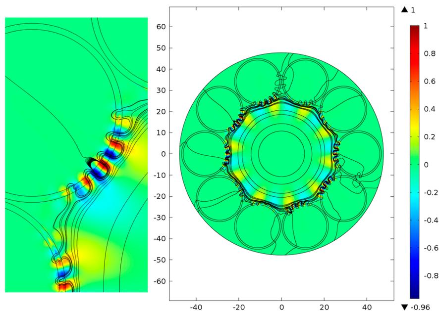
**Figure 5.** Distribution of the transverse Poynting vector component projection on the radius vector direction in the cross section of a silica glass negative curvature hollow core fiber (NCHCF) with ten very closely located cladding capillaries. The streamlines for the transverse component of Poynting vector (black lines).
