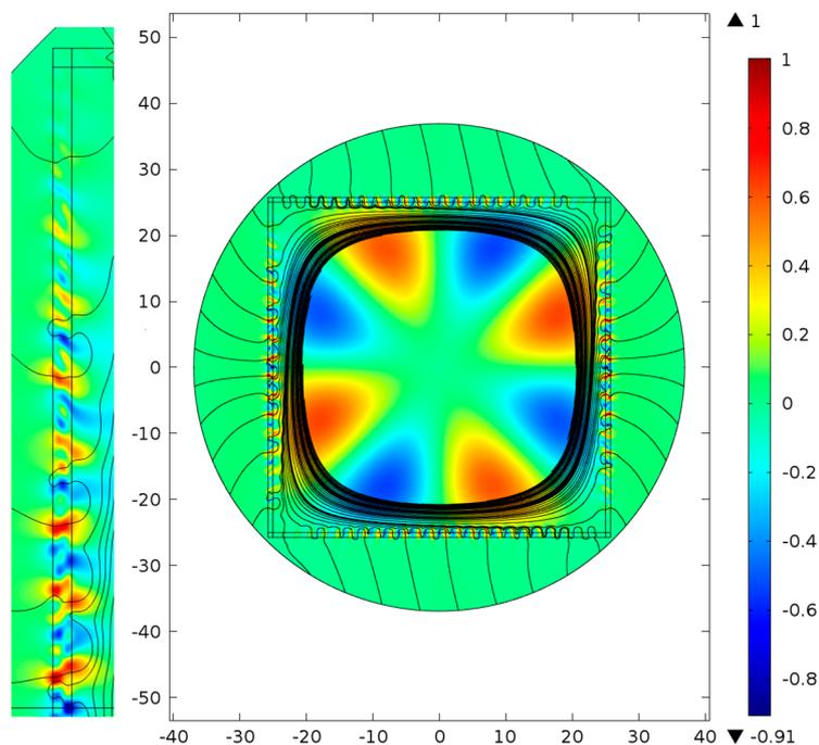
**Figure 4.** Distribution of the transverse Poynting vector component projection on the radius vector direction in the silica glass square waveguide microstructure cross section. The streamlines for the transverse component of Poynting vector (black lines).
