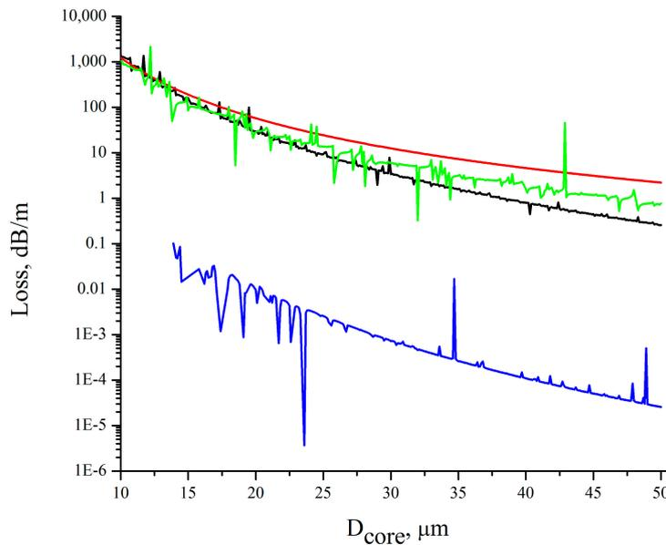
**Figure 1.** Waveguide loss dependence on the value of the air core diameter for a silica glass capillary (red), a silica glass octagon waveguide (green), a silica glass square waveguide (black), and a silica glass negative curvature microstructure with ten capillaries in the cladding (blue).
