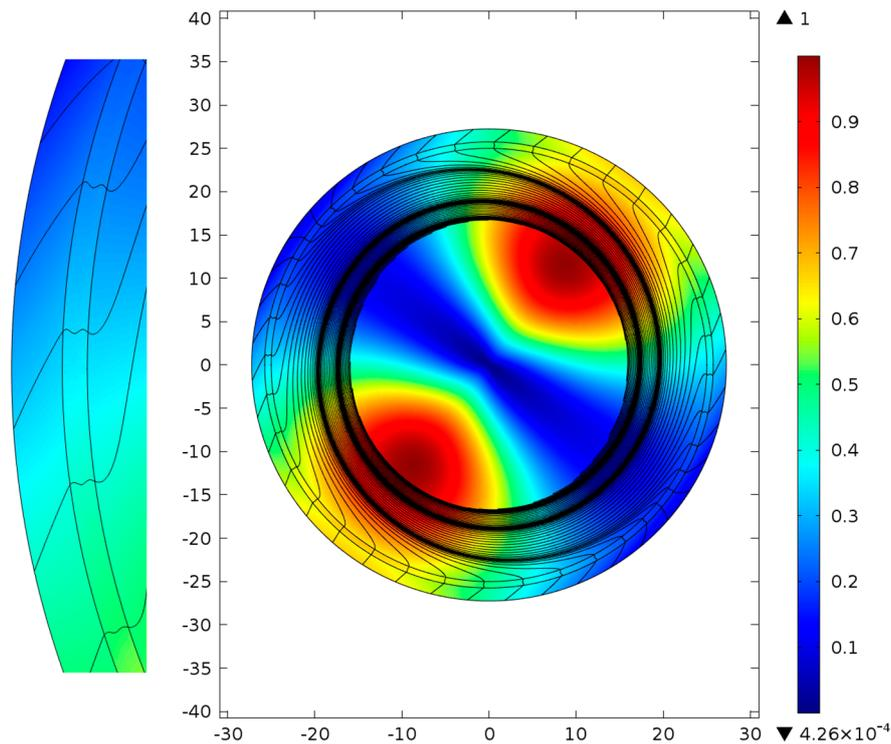
**Figure 2.** Distribution of the transverse Poynting vector component projection on the radius vector direction in the silica glass capillary cross section. The streamlines for the transverse component of Poynting vector (black lines).
