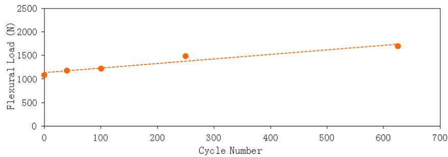
**Figure 9.** Maximum flexural loads vs. cycle numbers for the control specimens. Each cycle is equivalent to 2 h.
