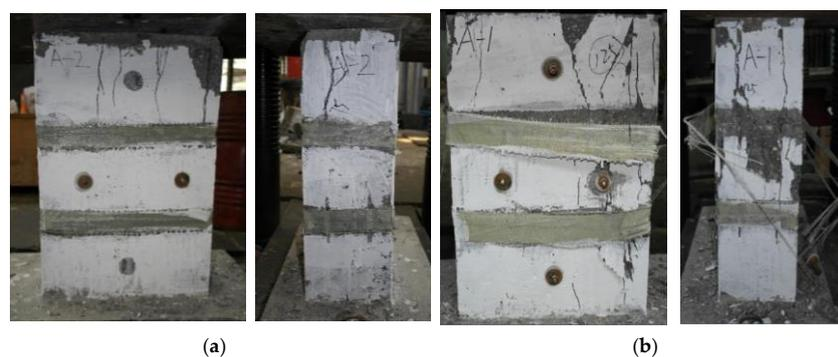
**Figure 5.** Compressive failure modes of the G-GMM specimen: (a) failure mode of the masonry; (b) failure mode of glass fiber-reinforced polymer (GFRP).
