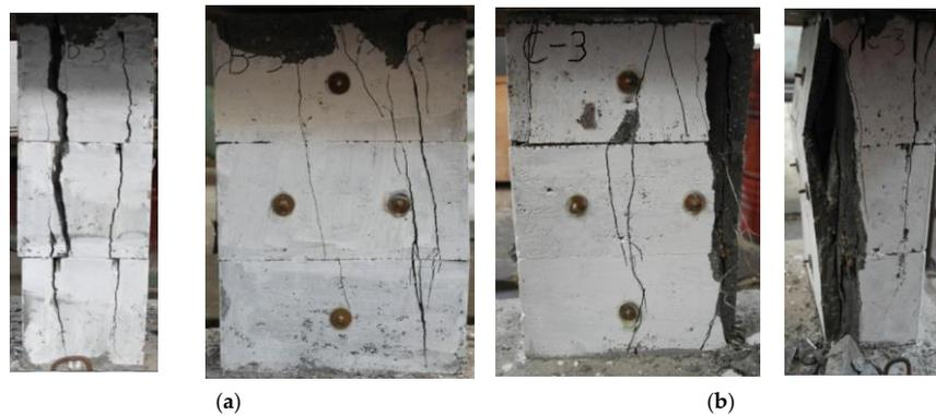
**Figure 4.** Typical compressive failure modes of the unstrengthened specimens: (a) failure mode 1 (Specimen B-3); (b) failure mode 2 (Specimen C-3).
