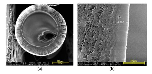
**Figure 11.** SEM micrographs: (**a**) the hollow fiber cross section; (**b**) PTMSP selective layer on the porous PSf support modified by air plasma (cross section fragment).
