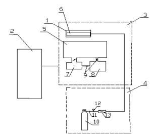
**Figure 2.** Functional diagram of the pilot scale setup for hollow fibers modification. 1—plasmatron; 2—HF generator; 3—vacuum module; 4—gas supply system; 5—shutter; 6—hollow fiber membrane; 7—diffusion pump; 8—forvacuum pump; 9—valves; 10—gas pressure tank; 11—reducing valve; 12—standard pressure gauge; 13—variable area flow meter.
