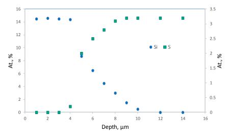
**Figure 12.** Atomic Si and S fraction dependence on composite PTMSP/PSf membrane selective layer scanning depth. The curve is obtained by EPMA technique.
