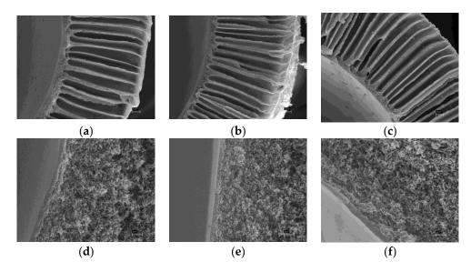
**Figure 6.** Image segment of the hollow fiber cross section,  $350 \times$  magnification: (a) virgin membrane; (b) air plasma treated membrane; (c) piranha mixture treated membrane; image segment of the fiber cross section: selective layer + transition layer part,  $20,000 \times$  magnitude: (d) virgin membrane; (e) air plasma treated membrane; (f) piranha mixture treated membrane.
