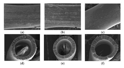
Figure 5. Image segment of the fiber outer surface,  $100 \times$  magnification: (a) virgin membrane; (b) air plasma treated membrane; (c) piranha mixture treated membrane; fiber cross section image,  $130 \times$  magnification: (d) virgin membrane; (e) air plasma treated membrane; (f) piranha mixture treated membrane.
