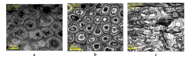
**Figure 10.** Hollow fiber membrane outer surface microrelief: (**a**) reference sample; (**b**) membrane treated by air plasma; (**c**) membrane treated by piranha mixture ( $2000 \times$  magnification).
