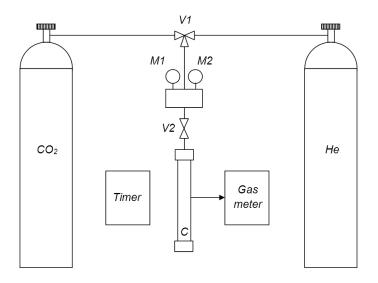
Figure 4. Functional diagram of the laboratory setup for membranes gas permeance measurement.
