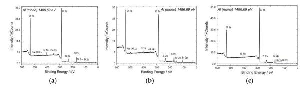
**Figure 8.** XPS spectra: virgin PSf membrane (**a**); PSf membrane surface after air plasma treatment (**b**); PSf membrane surface after piranha mixture treatment (**c**).
