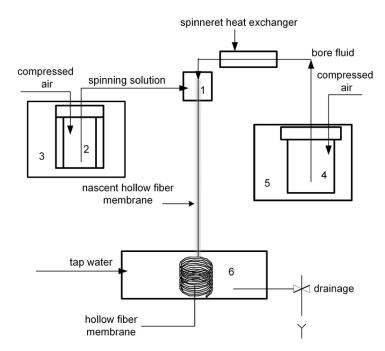
**Figure 1.** Functional diagram of the setup used for spinning of hollow fiber membranes. 1—spinneret; 2—tank for the spinning solution; 3—thermostat; 4—tank for the bore fluid; 5—thermostat; 6—coagulation bath.
