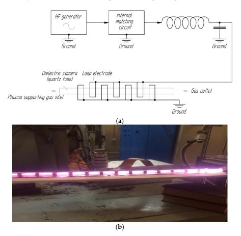
**Figure 3.** (a) Gas discharge chamber electrode connection diagram; (b) Experimental gas discharge chamber for hollow fiber membranes treatment.
