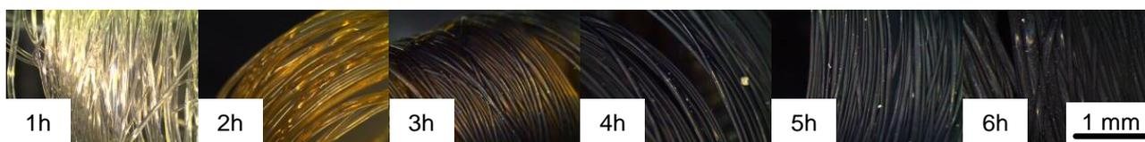
**Figure 2.** Color change of sample P-PE-HDPE-41 (crystallinity: 66%, single filament diameter 16.4  $\mu\text{m}$ ).
