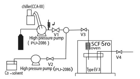
Figure 2. Supercritical CO<sub>2</sub> apparatus.
