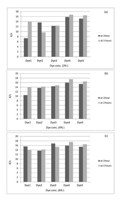
Figure 7. (a) Effect of dyeing time at 2% dye conc; (b) at 4% dye conc; (c) at 6% dye conc.
