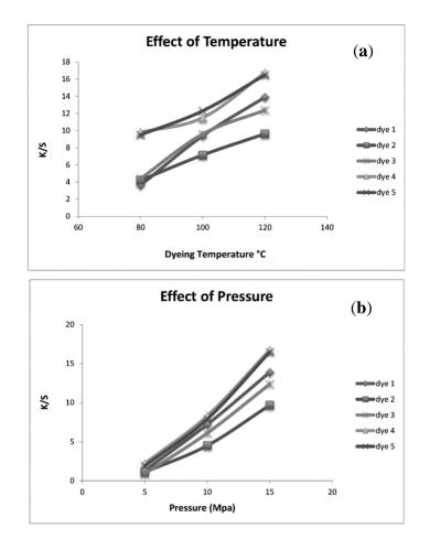
Figure 6. (a) Effect of dyeing temperature; (b) Effect of dyeing pressure.
