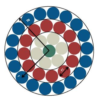
Figure 4. Ideal packing of circular fibers in yarns.
