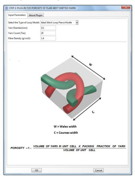
Figure 6. Plug-in for porosity of plain weft knitted fabric.
