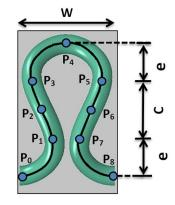
Figure 2. Geometry of a plain weft knitted loop.
