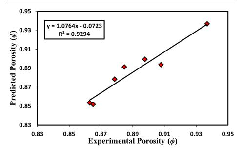
Figure 8. Comparison of porosity between plug-in predicted and experimental.
